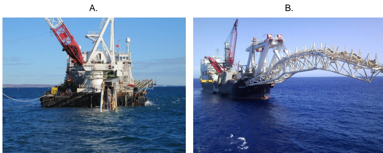
Figure 2-4: Examples of A. shallow water lay barge and B. a conventional pipelay vessel
