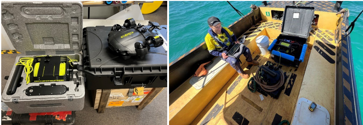
Plate 2-1 ROV with deck power supply (left) and set up on deck (right)
