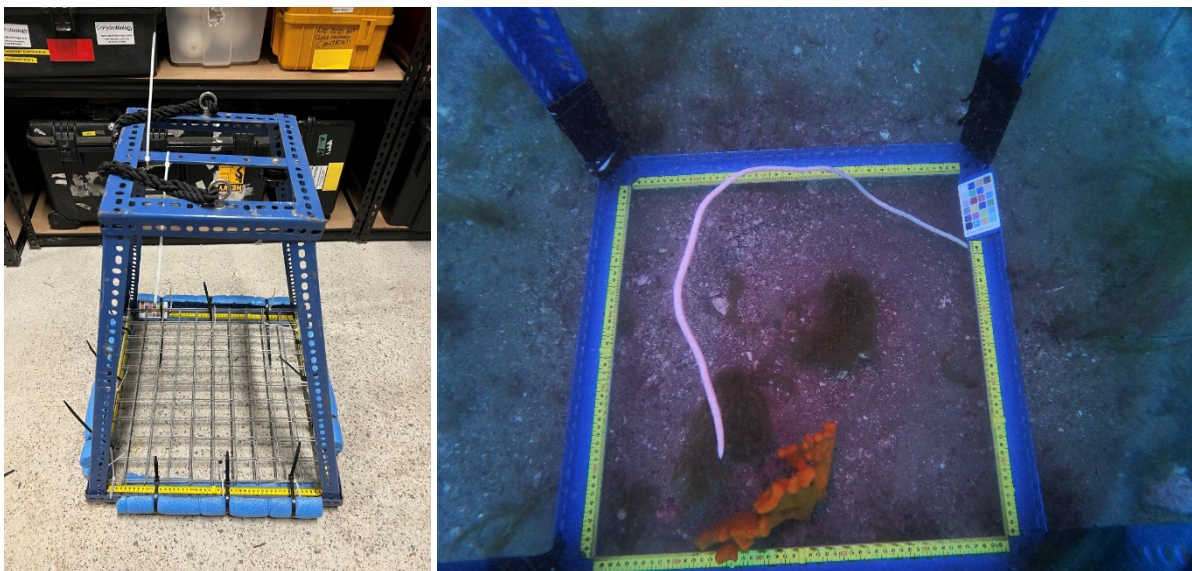
Plate 2-2 Drop camera frame system with 50 x 50 cm quadrat (left) In water use (right)
