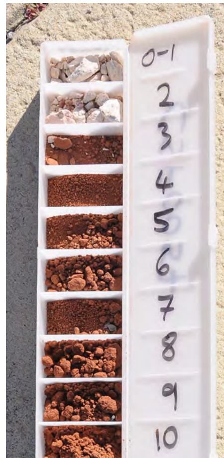
TYPE T3 Coarse-grain channel fill representative of paleochannels
