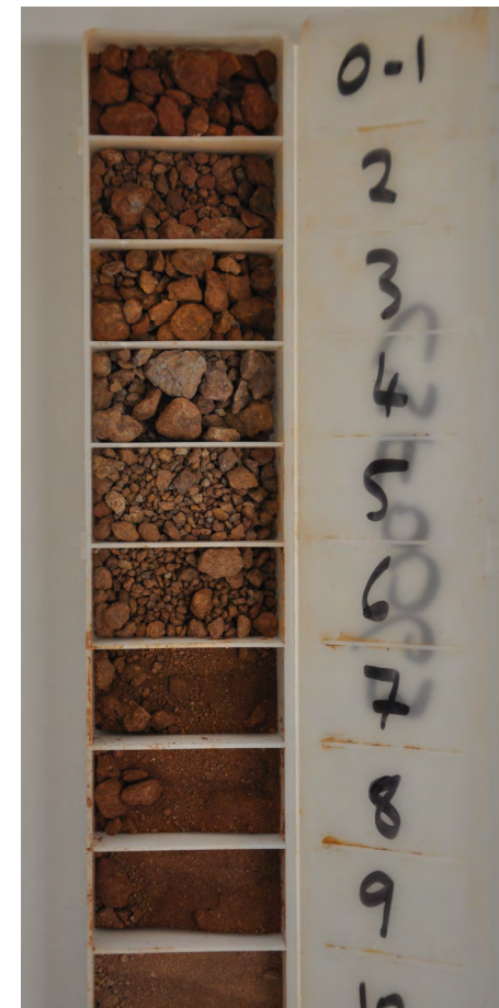
TYPE T4 High sand and silt content (saprolite)
