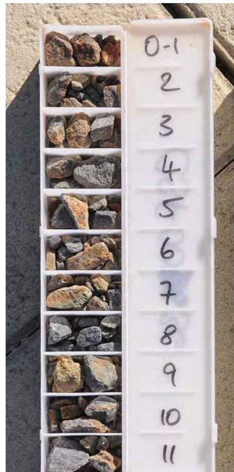
TYPE T2 Weathered and highly fractured basement (saprock)
