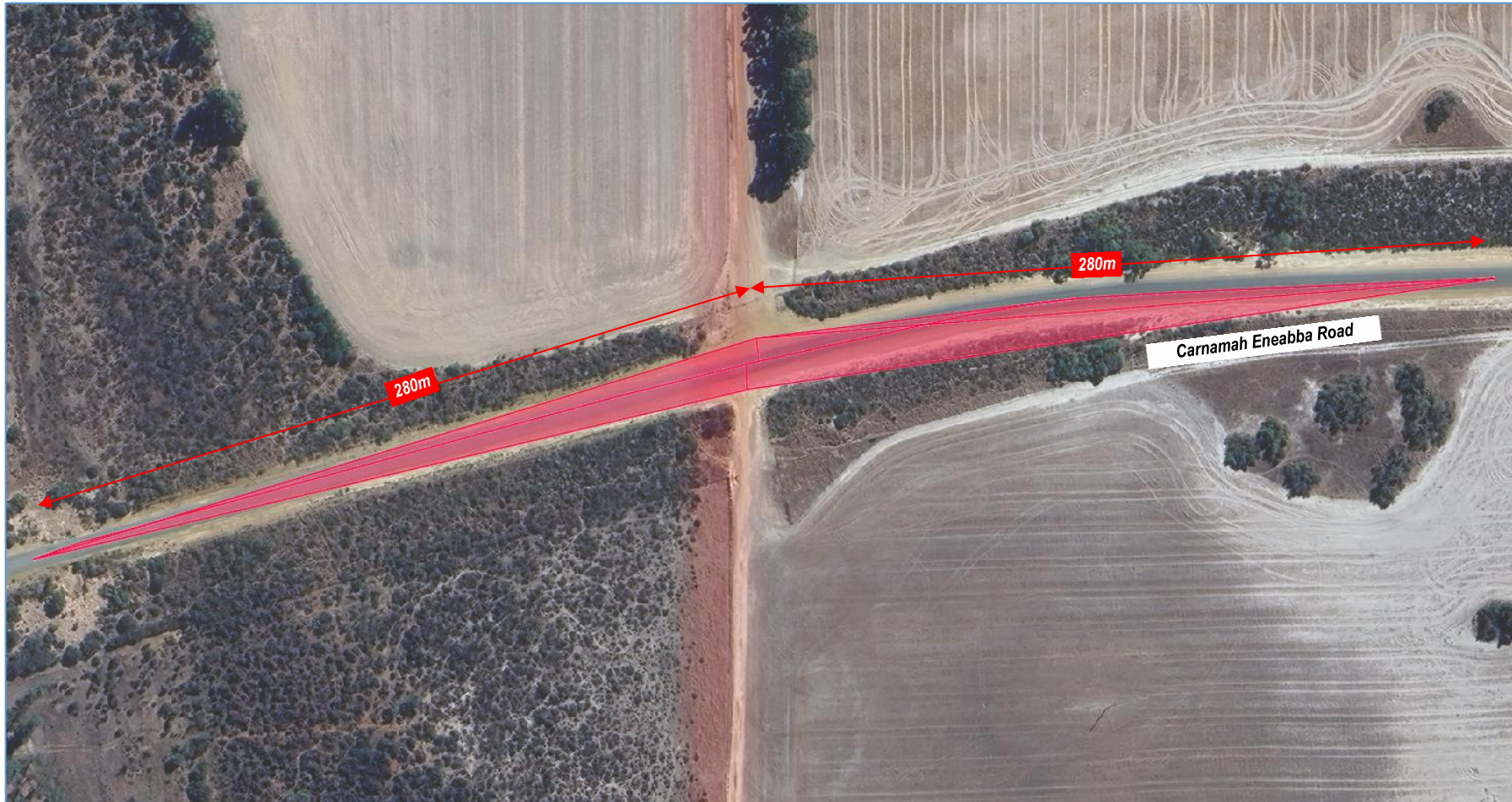
Figure 11: Sight Distance Check – Access 2 on Carnamah Eneabba Road
