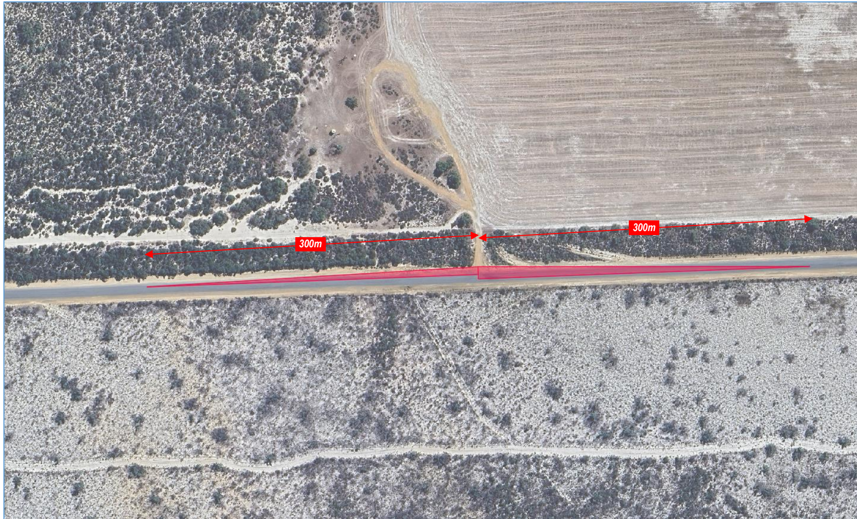
Figure 14: Sight Distance Check – Access 5 on Carnamah Eneabba Road
