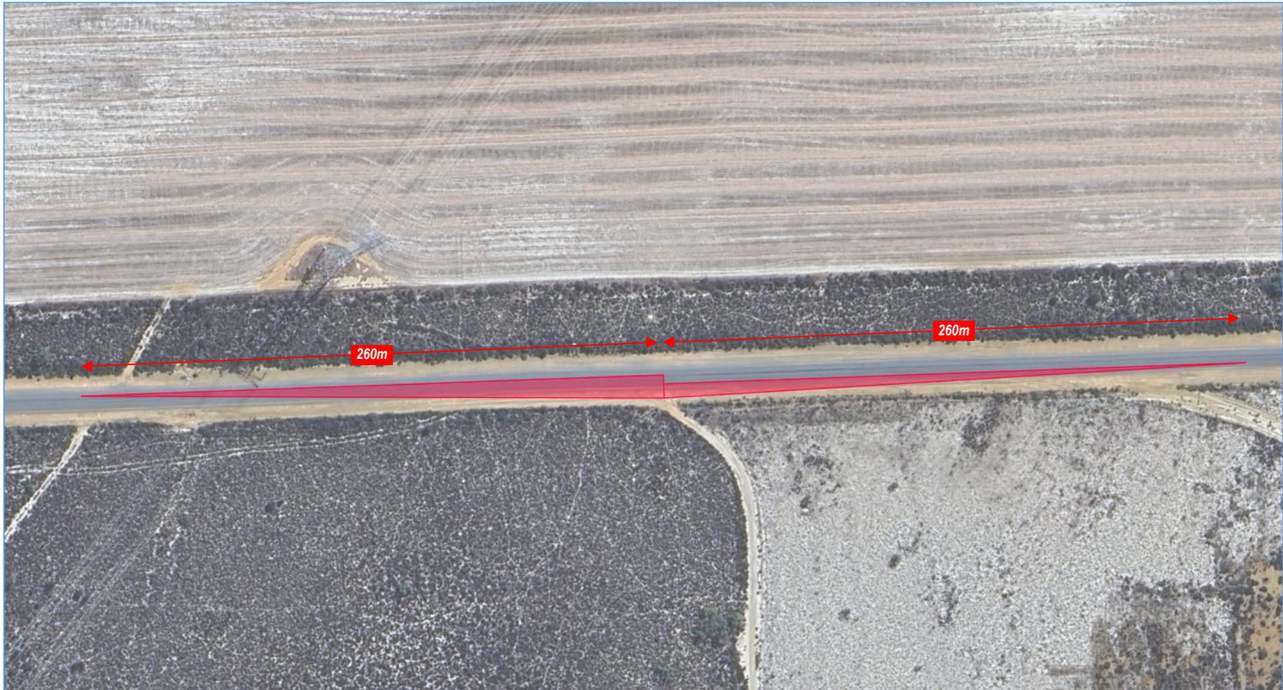
Figure 13: Sight Distance Check – Access 4 on Carnamah Eneabba Road
