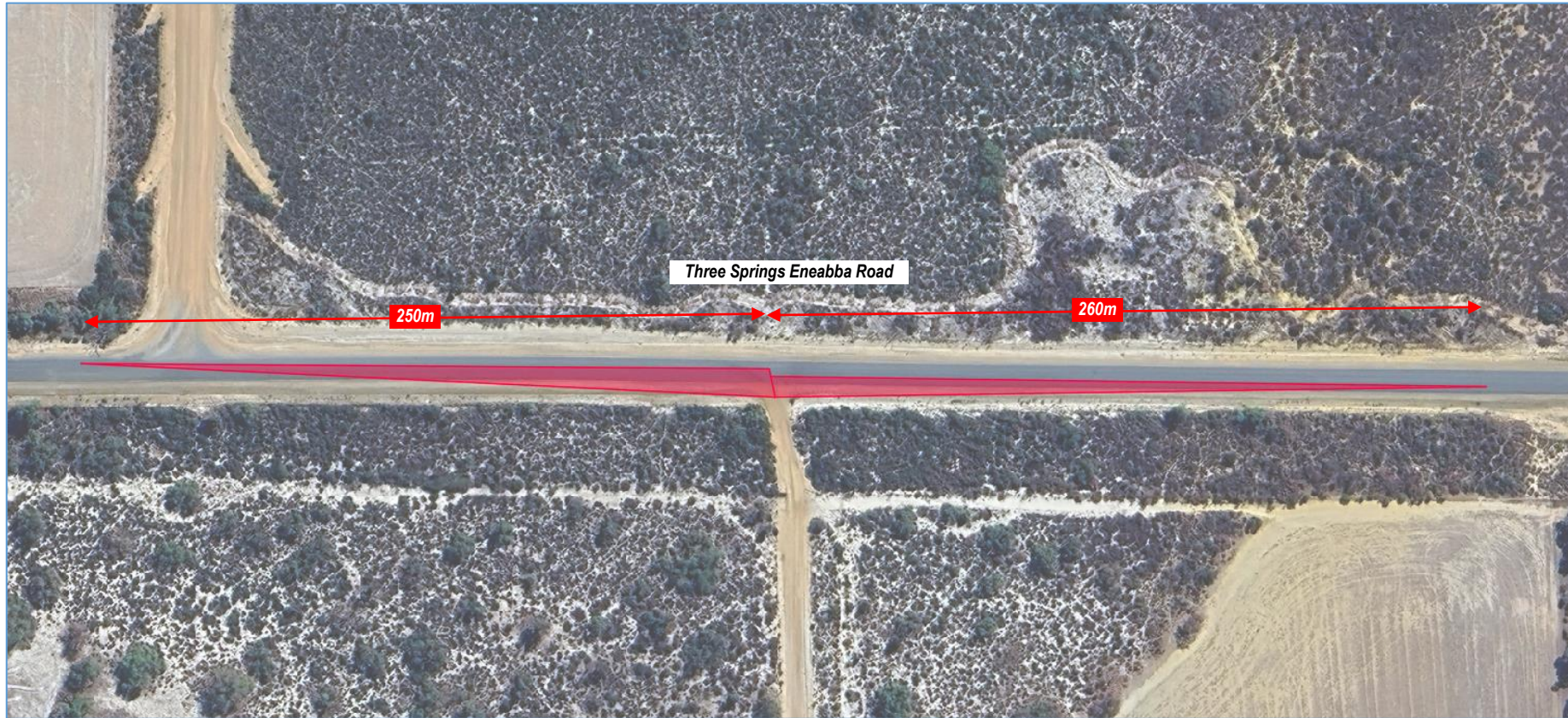
Figure 10: Sight Distance Check – Access 1 on Three Springs Eneabba Road
