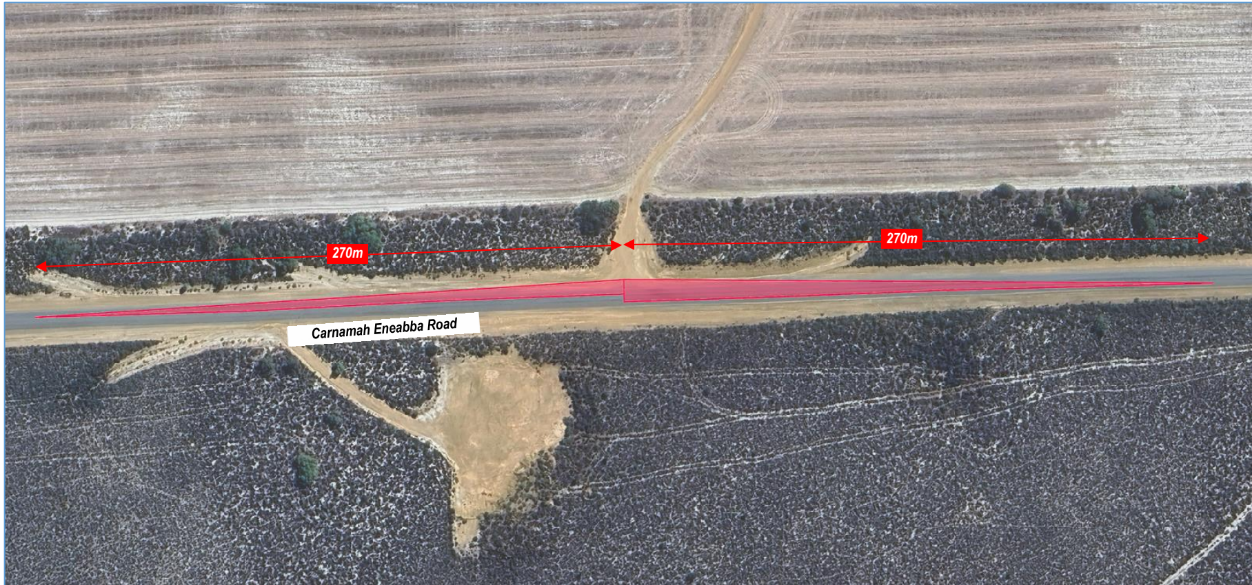
Figure 12: Sight Distance Check – Access 3 on Carnamah Eneabba Road
