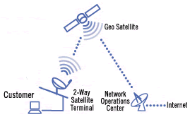
Two-way connection to the internet via satellite [35]
