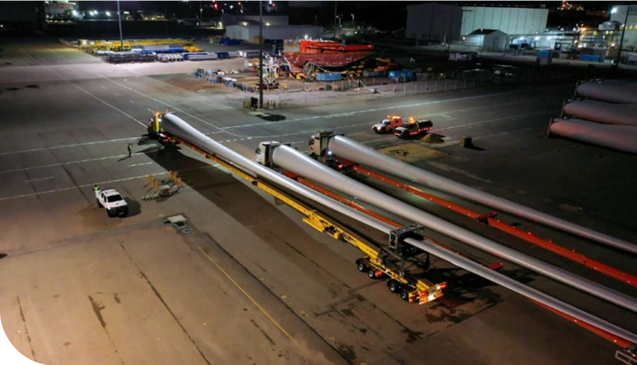
Above: Extendable blade trailers loaded with 75m blades for the Yandin project in Western Australia.
