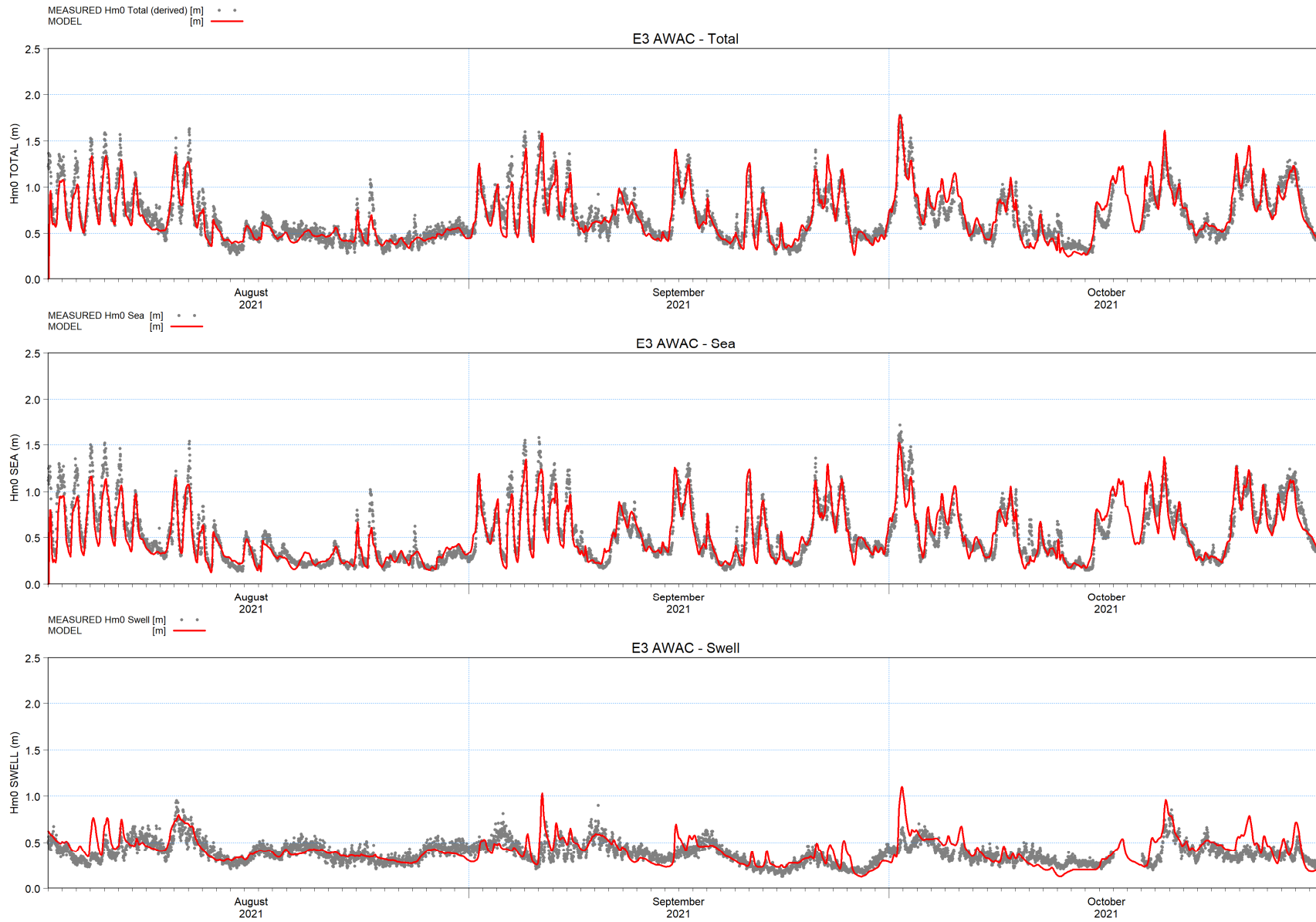
Figure B-3 Time series comparison for Local Wave Model hindcast vs. measured Hm0 (Total, Sea, Swell). Station E3 AWAC, 2021.
