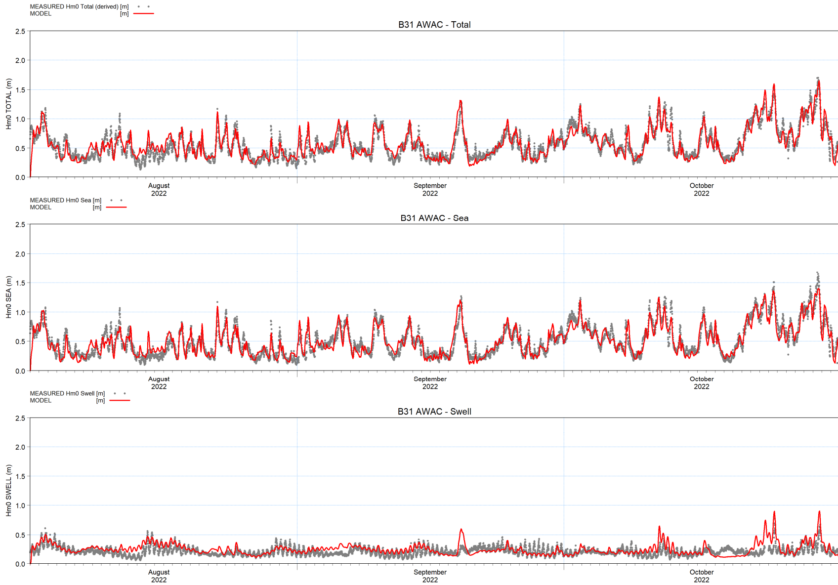
Figure B-10 Time series comparison for Local Wave Model hindcast vs. measured Hm0 (Total, Sea, Swell). Station B31 AWAC, 2022.
