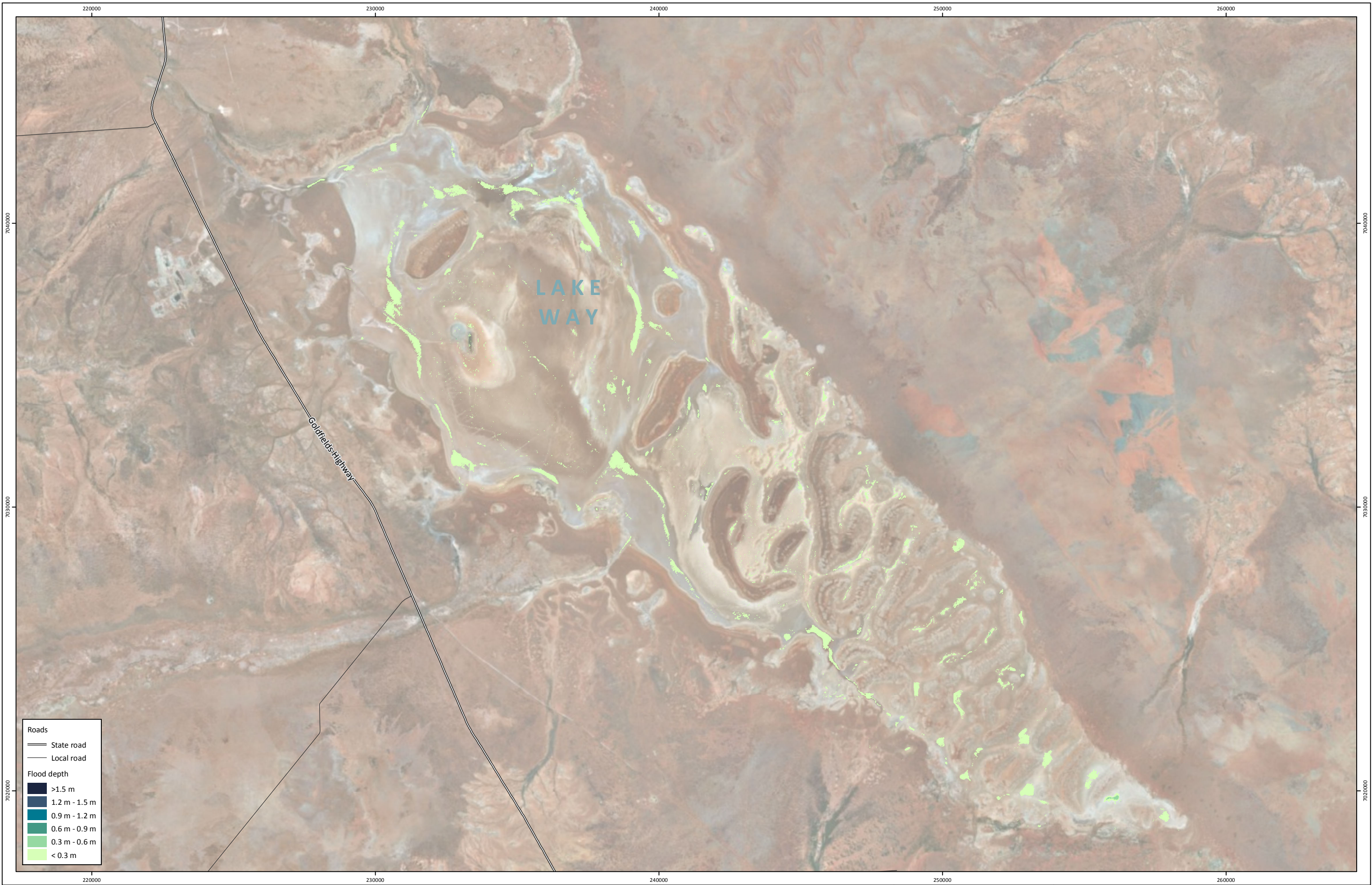
Figure 3: Pre-development 63.5% AEP Flood Inundation of Lake Way
