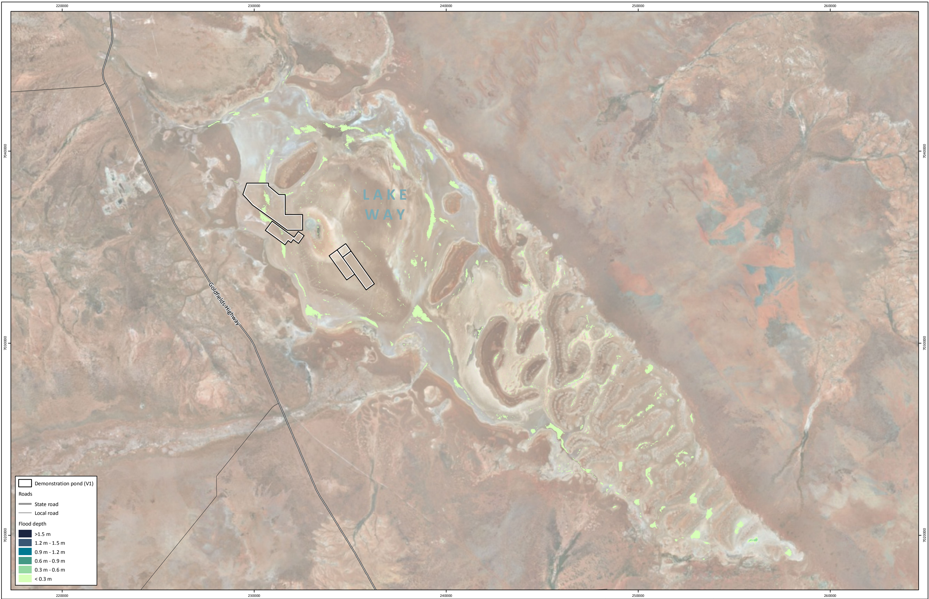
Figure 4: Post-development (Demonstration) 63.5% AEP Flood Inundation of Lake Way
