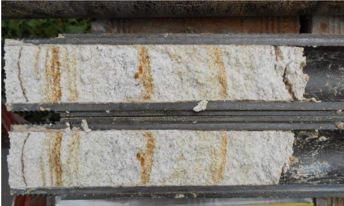
Photograph 2: Borehole DD05, SPT split spoon sampler at 15.1 m depth, showing thin orange brown sandy clay laminations within cream, clayey silty fine to medium sand.
