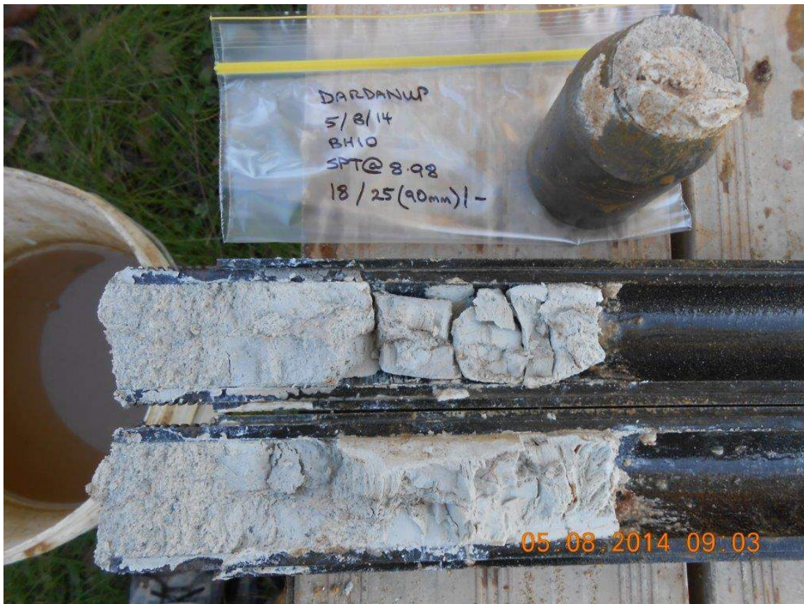
Photograph 3: Borehole DD10, SPT split spoon sampler at 9.0 m depth, showing 15 cm thick band of cream clay within clayey silty fine to medium sand matrix
