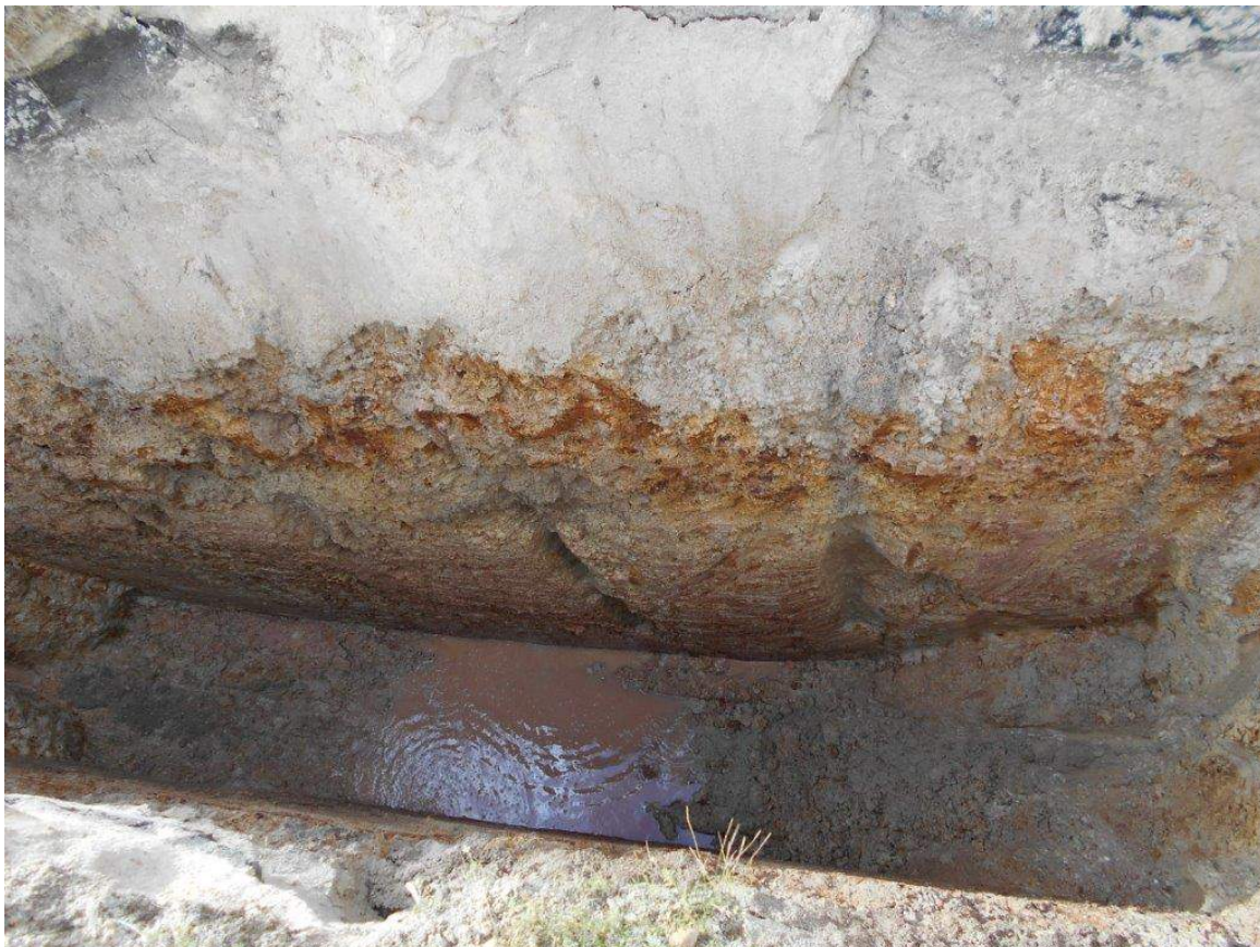
Photograph 1: Test Pit 24, located at 72 mAHD, showing the succession of colluvial/Aeolian sand over laterite then laterised clayey sand of the Yoganup formation.
