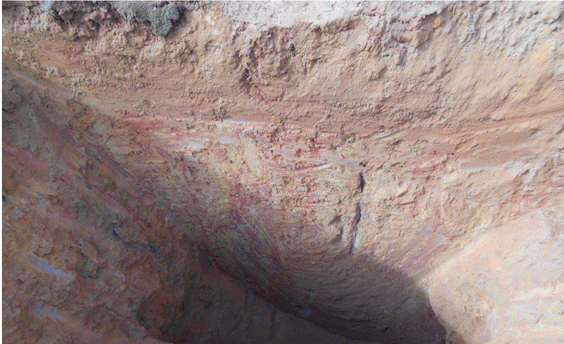
Photograph 4: Test Pit 40, located at 87 mAHD, showing hard, laterised red brown mottled orange brown and light grey, sandy CLAY/clayey SAND.
