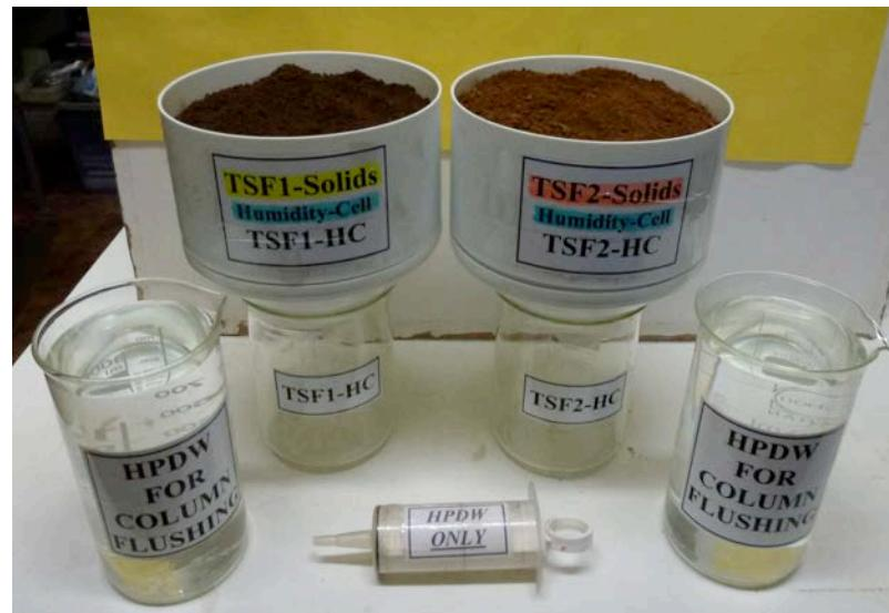
1.3 kg of HPDW was initially added to each HC as a pre-rinsing step, and the leachates collected in 1 L glass beakers.
