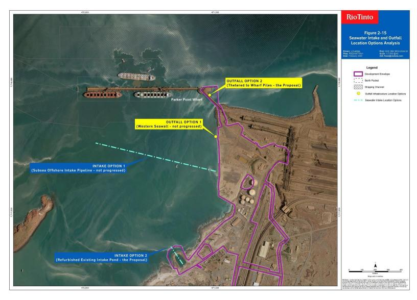
Figure 2-15: Seawater intake and outfall location options
