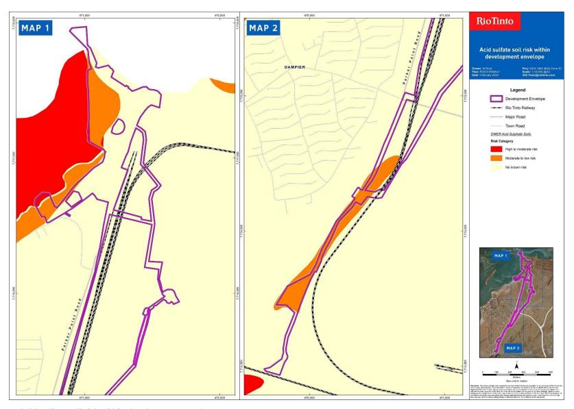
Figure 11-8: Acid sulfate soil risk within development envelope
