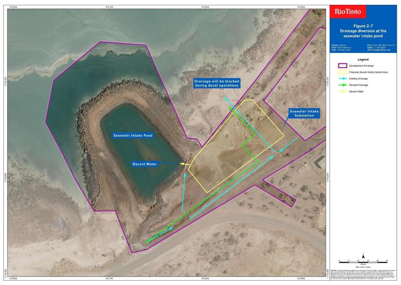
Figure 2-7: Drainage diversion at the seawater intake pond
