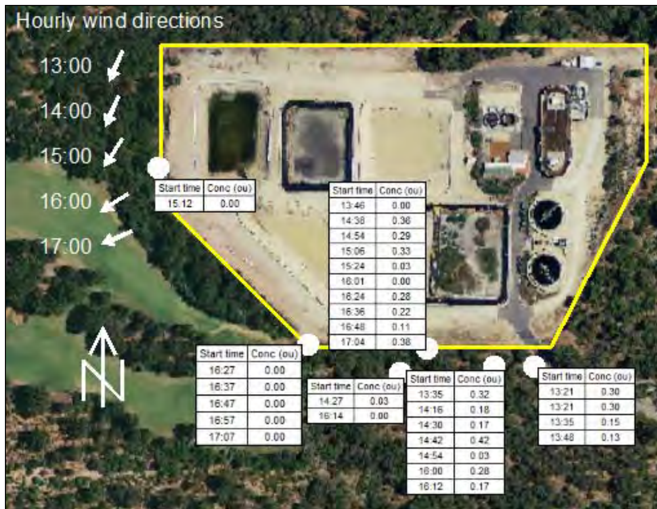
Figure 9 Estimated 10-minute average odour concentrations for each assessment 7/6/2014 and wind directions
