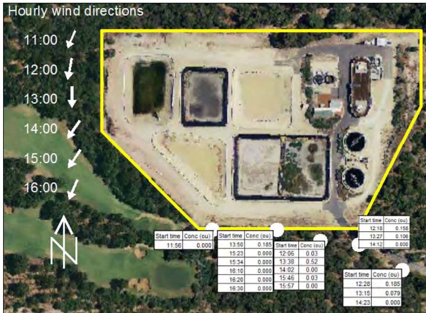
Figure 8 Estimated 10-minute average odour concentrations for each assessment 31/5/2014 and wind directions
