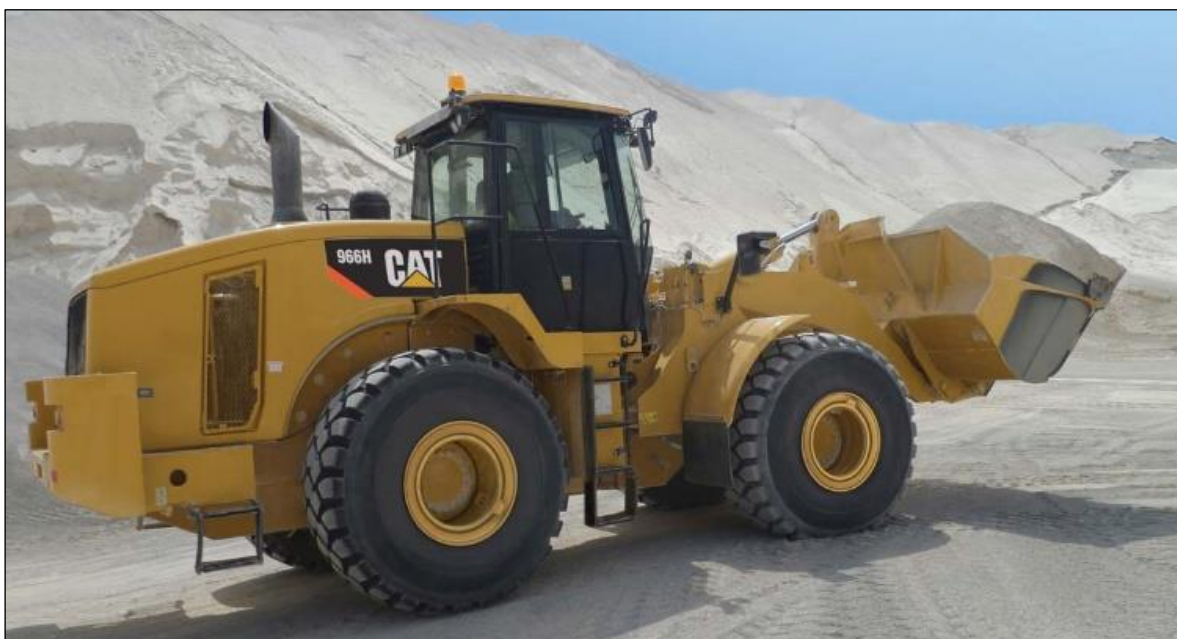
Plate 2-1 50-tonne Operating Weight Front End-Loader for Excavation
