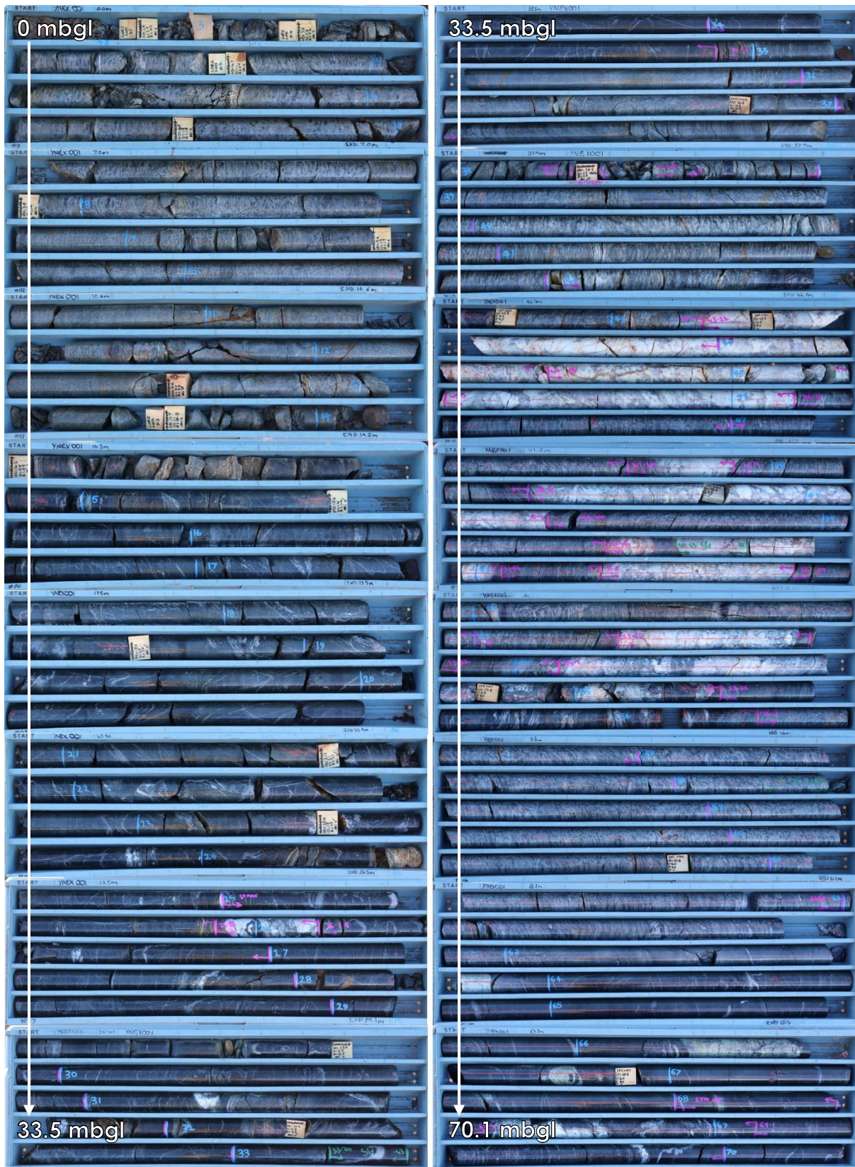
Figure 4-9: Diamond drill core images (0–70.1 mbgl) of YNEX001, located within proposed pit area, 150 m west of YRRD025 (recorded SWL ranged from 17.4 to 18.8 mbgl), from which stygofauna were recorded.
