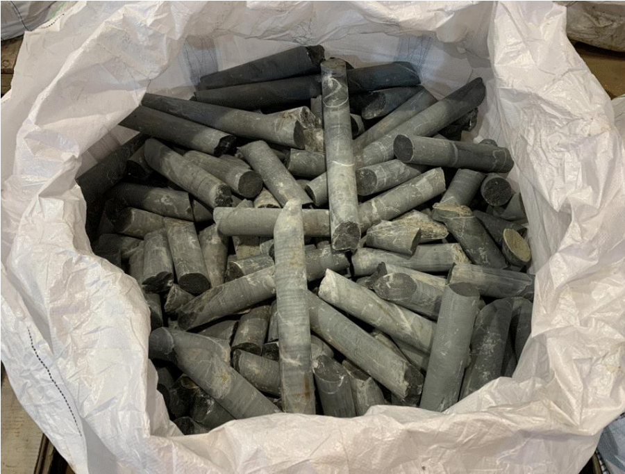
Plate 3 Raw drill cores of amphibolite as received
