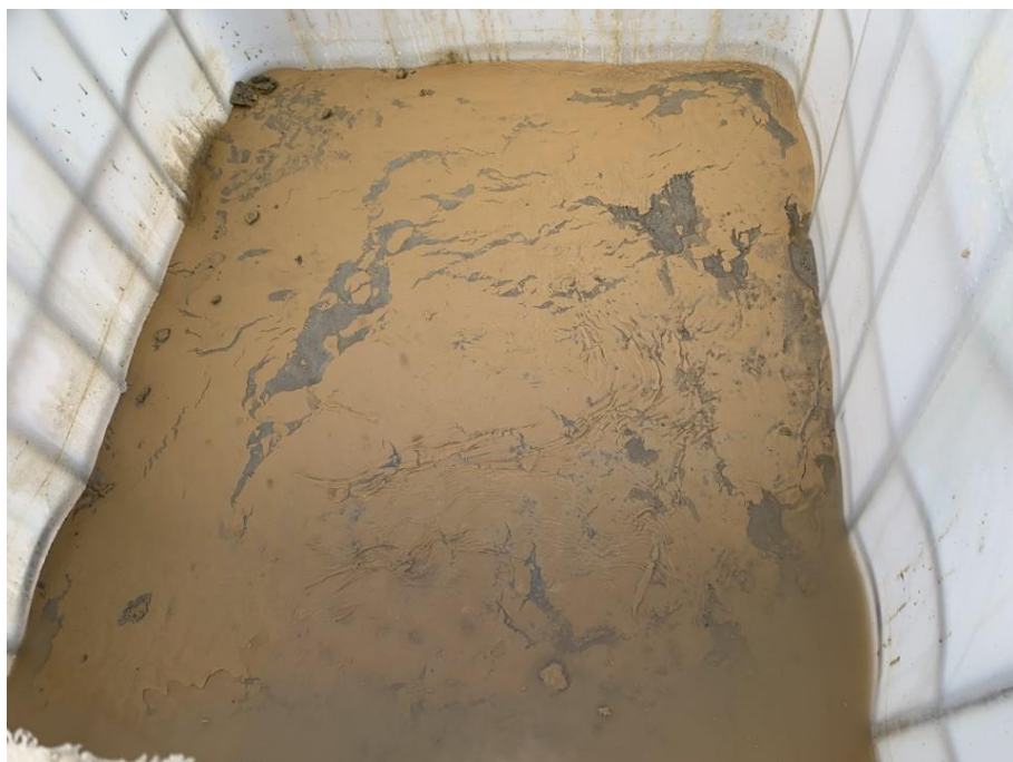
Plate 11 Raw tailing materials as received
