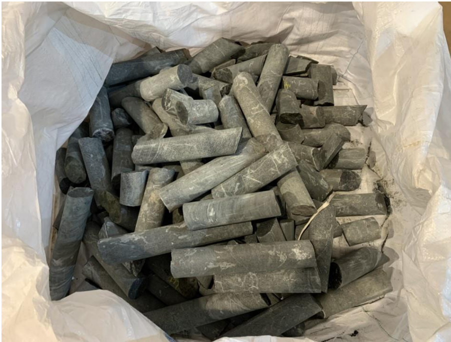
Plate 5 Raw drill cores of dolerite as received
