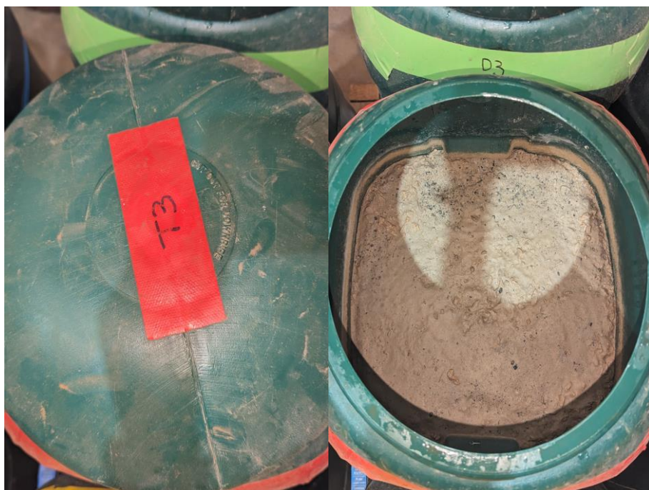
Plate 12 Equipment setup of leaching test for tailings
