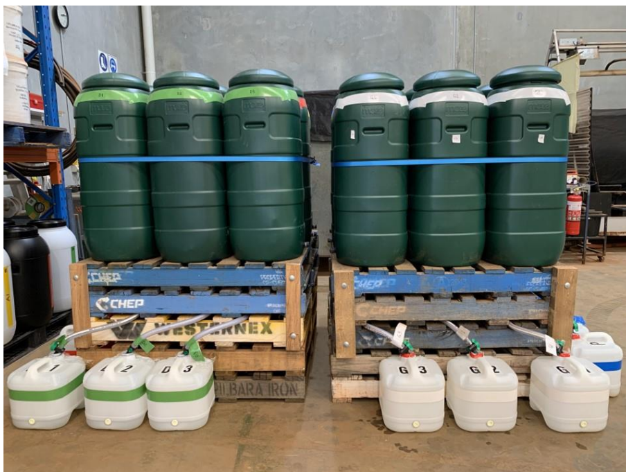
Plate 2 Kinetic leaching test set-up
