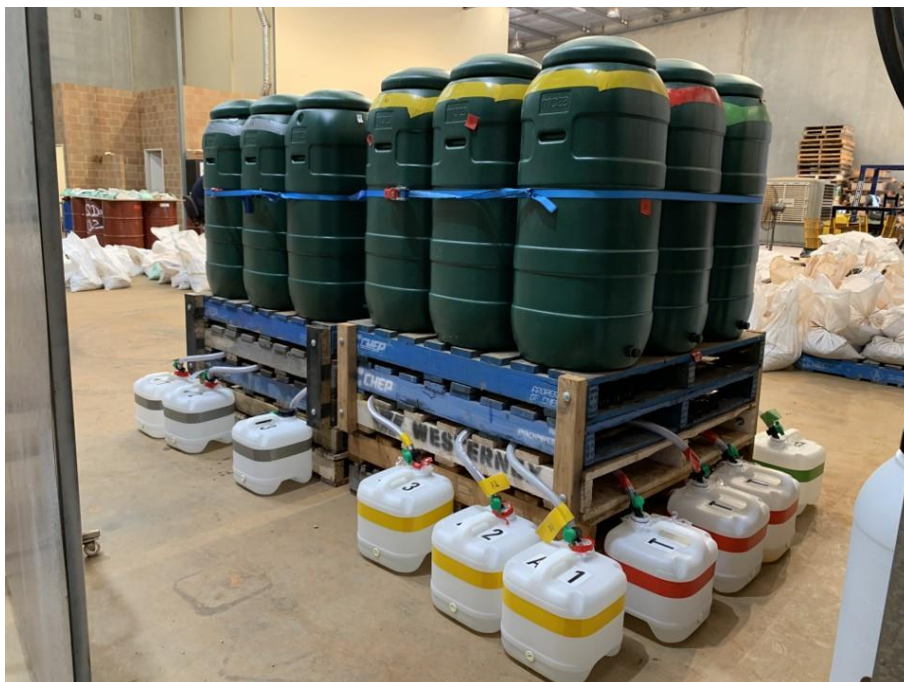
Plate 1 Kinetic leaching test set-up 1
