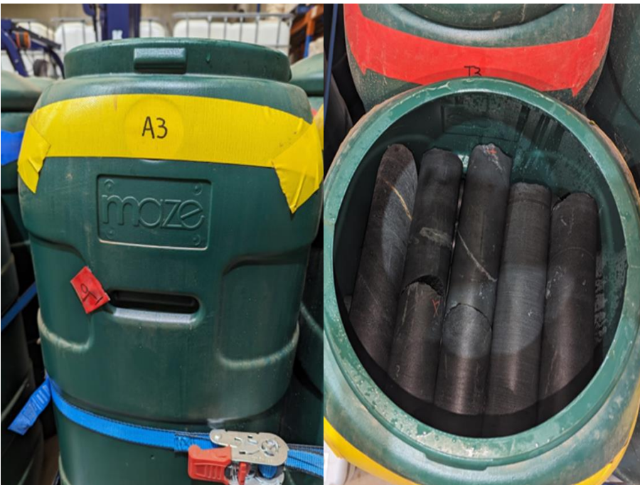
Plate 4 Equipment setup of leaching test for amphibolite
