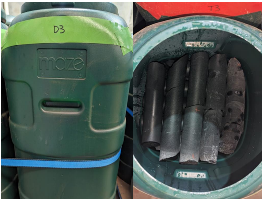
Plate 6 Equipment setup of leaching test for dolerite
