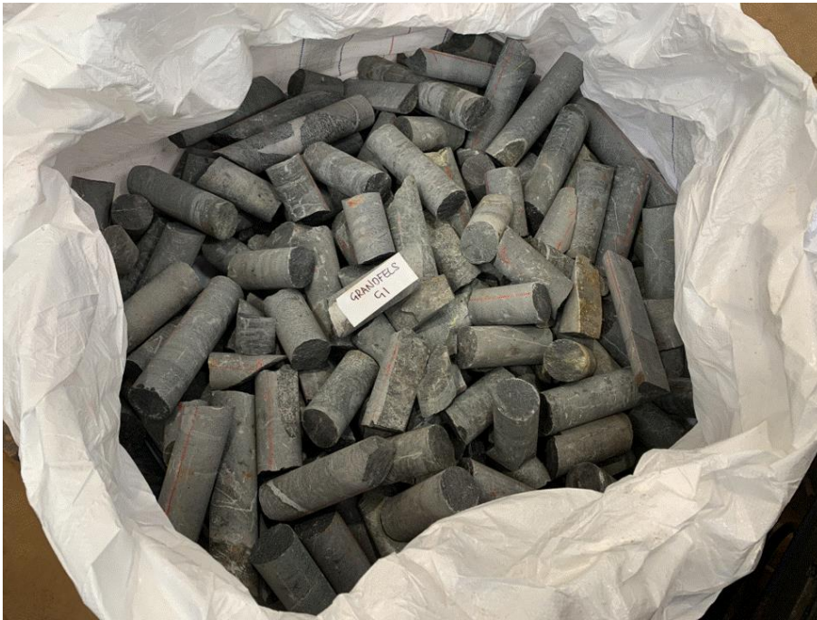
Plate 7 Raw drill cores of granofels as received
