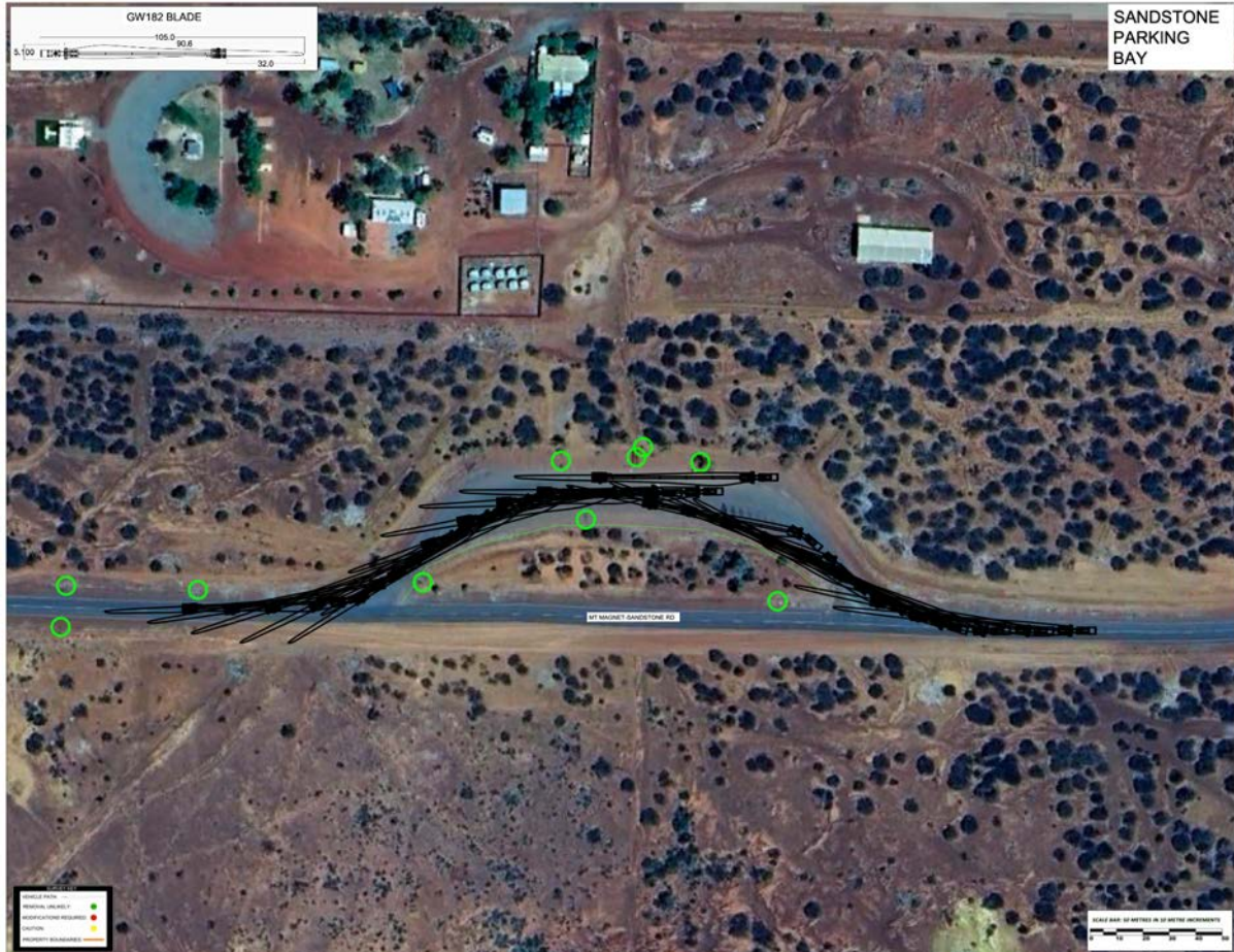
Image 15: Entering and exiting Sandstone parking bay.
