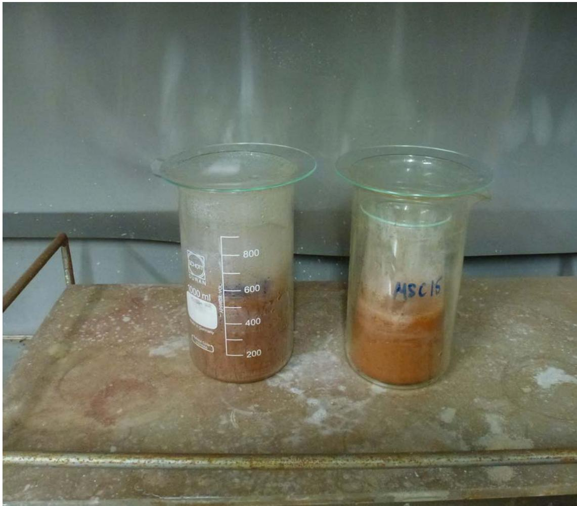
**NAG Testwork: 1st-Boiling Step [without Cu(II) addition] After Overnight Reaction**
