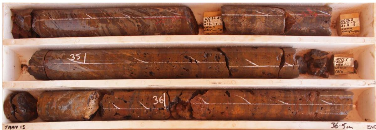
**Figure 18 Core photo of Chert from 34.0 – 36.5 m depth in MRDH0003**
