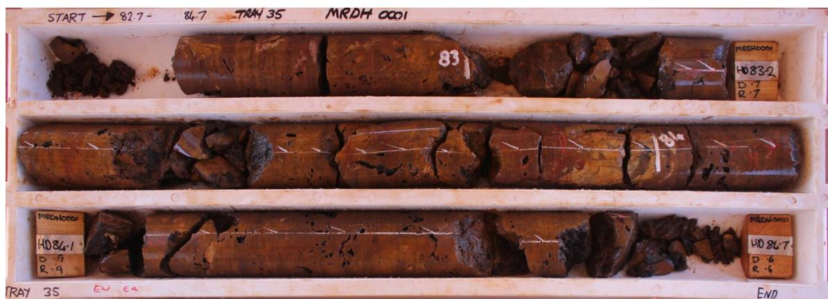
**Figure 17 Core photo of BIF from 82.7 – 84.7 m depth in MRDH0001**
