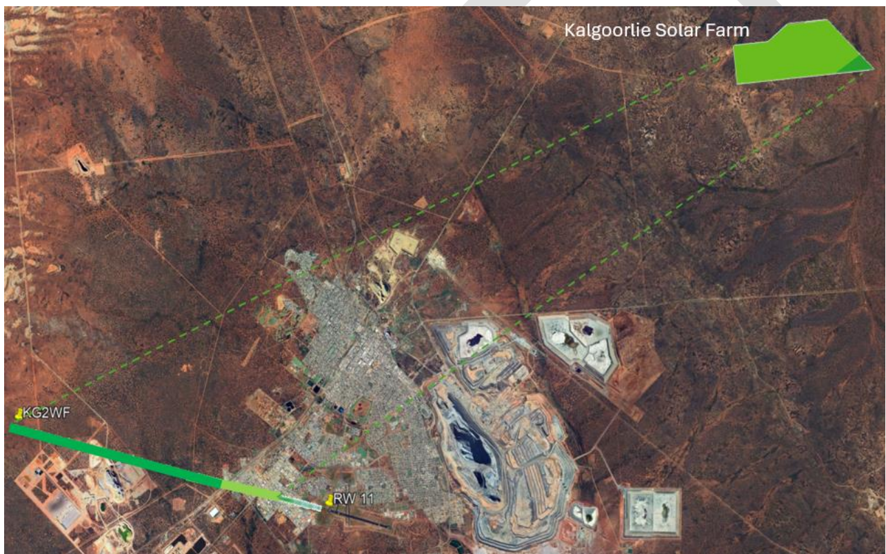
Figure 5.3 Predicted glare impact on RW 11 – fixed tilt, West
