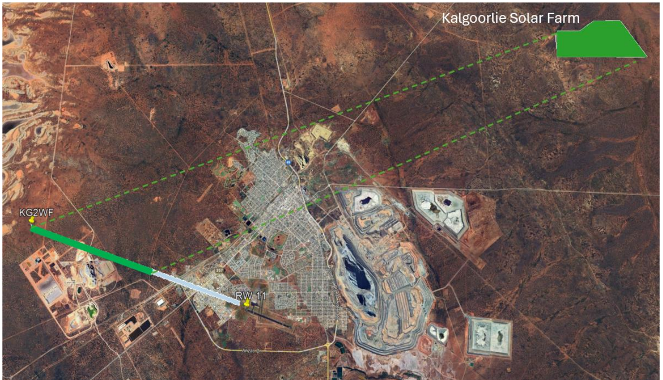
Figure 5.2 Predicted glare impact on RW 11 – backtracking ON
