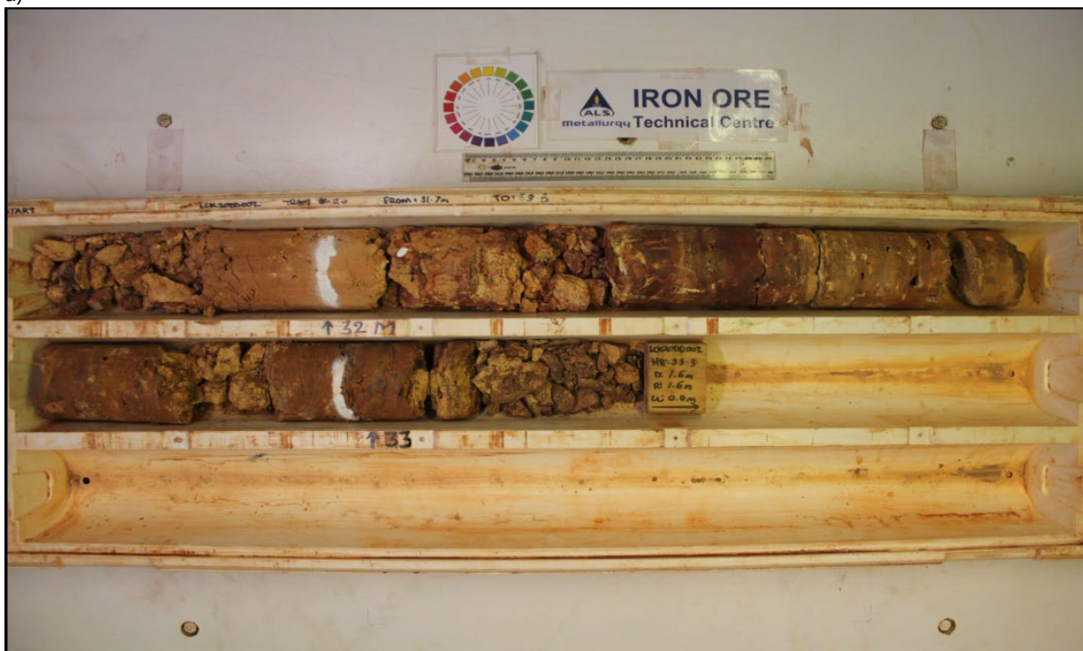
Figure 14: a) core from D4 Dales gorge sub member demonstrating weathering and subterranean spaces and b) core from D3 dales gorge sub member show clay and a lack of subterranean spaces.
