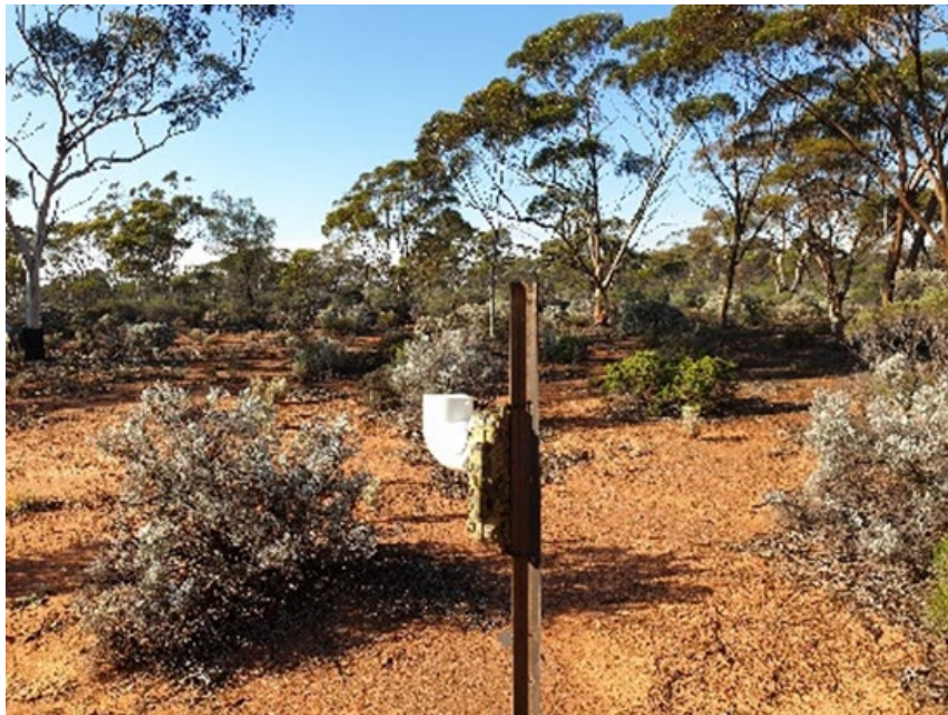
Figure 4. Ranger bat detector with directional microphone funnelling upwards
