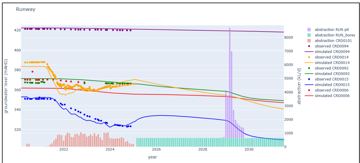
Figure 5.2: Current and simulated drawdown at Runway Pit
