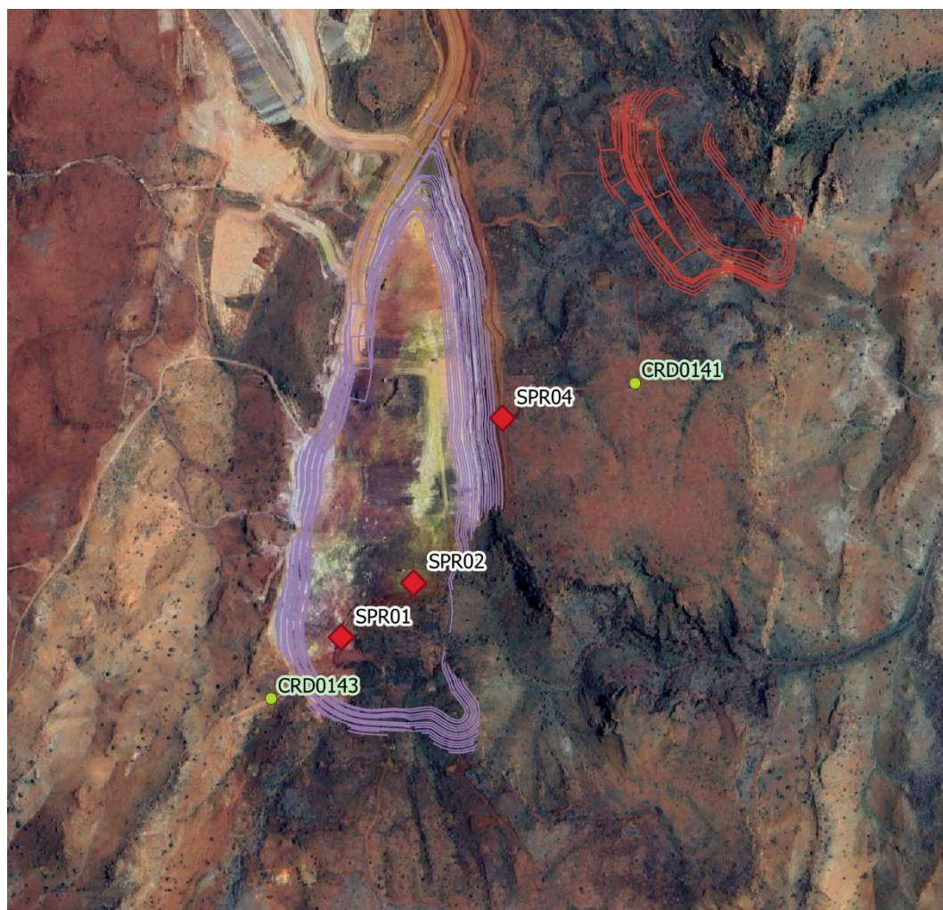
Figure E.5 Location of Sparrow Lake pit geotechnical bores used for packer test holes relative to production bores used in the 2024 pumping test results
