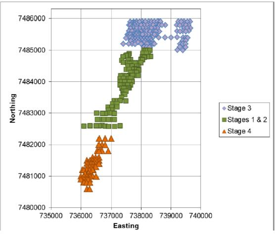
Figure 3: Collar locations for drillholes used in sulphur assessment
