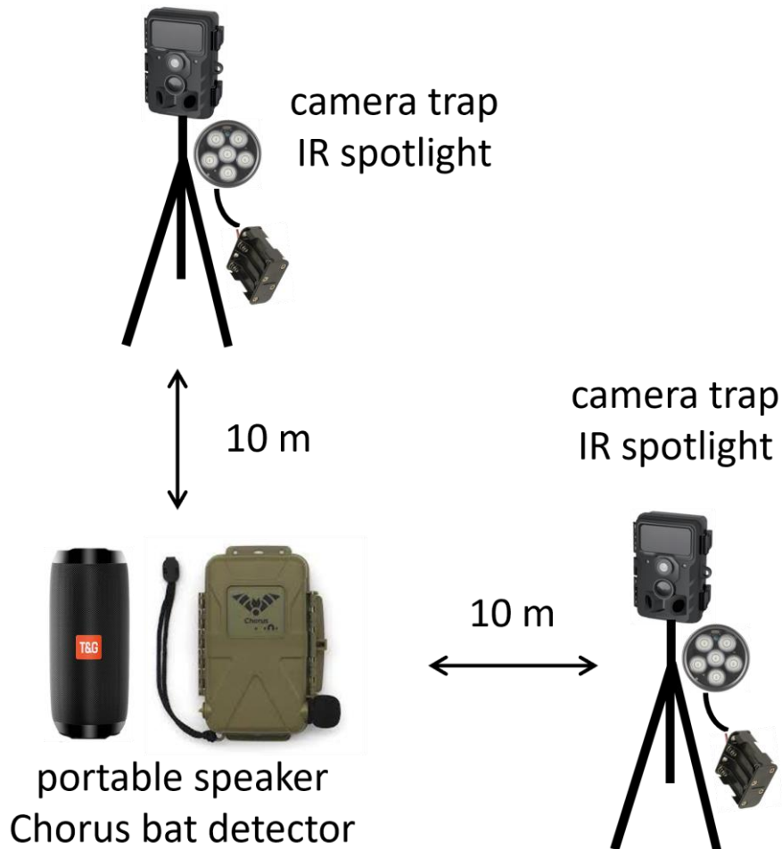
Figure 1. Representation of the acoustic lure system deployment. There are two camera traps for redundancy and corroboration of images of bats, and a bat detector for validation of an identification made from videos based on echolocation calls only.
