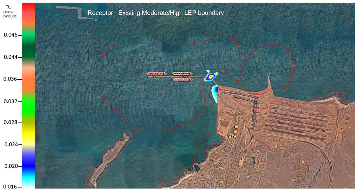
Figure 6-4 Modelled temperature difference results between case with outfall discharge and without outfall discharge (bottom water layer, winter): Scenario 1: 2°C above the ambient seawater temperature
