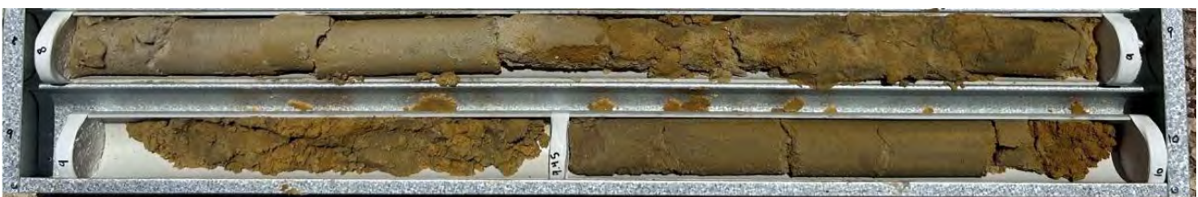
Figure 2: Tamala Sand – Residual Origin (BH141 10.0 – 12.0 m)
