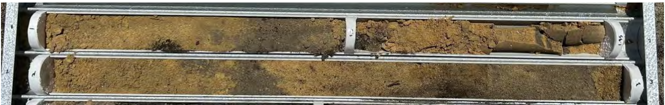
Figure 4: Fill Material (BH149 1.0 – 2.0m)
