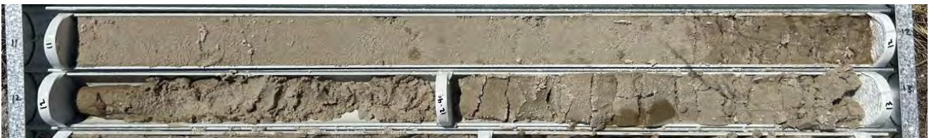
Figure 8: Bassendean Sand (BH37 11.0 – 13.0 m)
