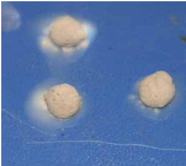
Re-moulded soil: Moderate dispersion at 2 minutes
