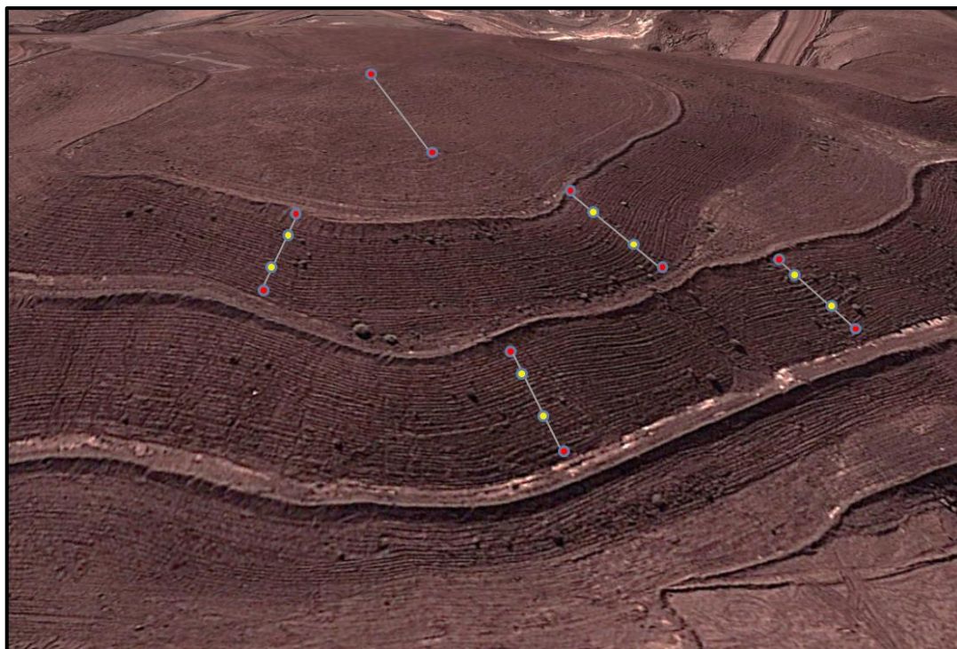
Figure 1: Example positioning of transects (50 m) on a rehabilitated waste dump, red markers indicate start and end posts and yellow markers indicated erosion posts
