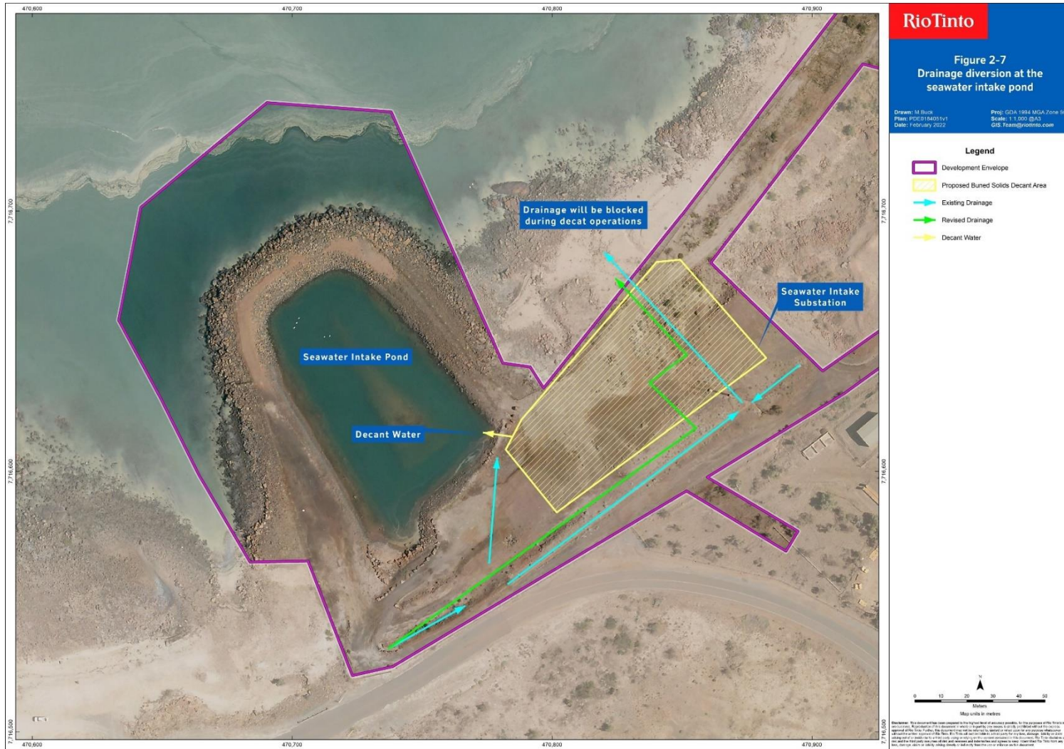
Figure 4: Drainage diversion at the seawater intake pond
