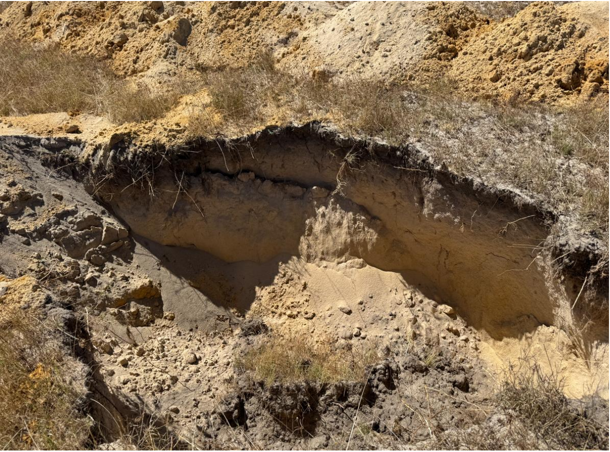
Figure 3: Soil profile of Test Pit 2 after cave in.
