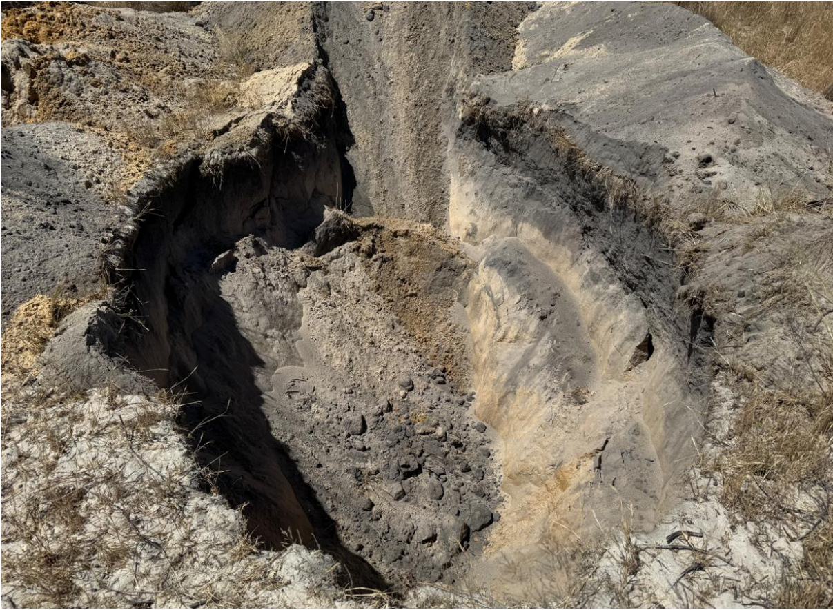
Figure 11: Soil profile of Test Pit 6.
