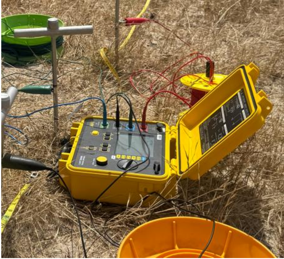
Figure 1: Earth resistivity tester used for investigations.
