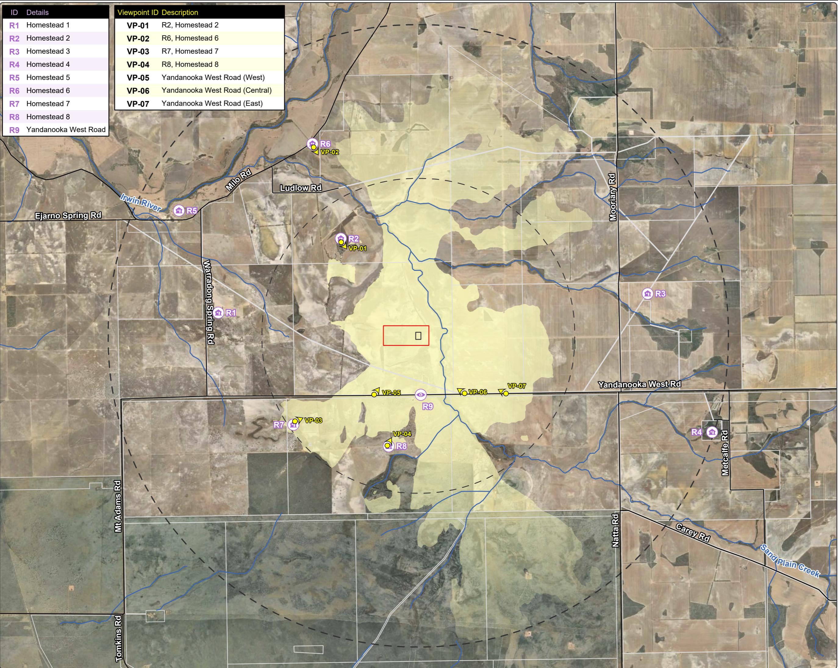
Figure 4-3 Wshed analysis: Gas Gensets (height 13.2m) and Still Column Tank (height 12m)
