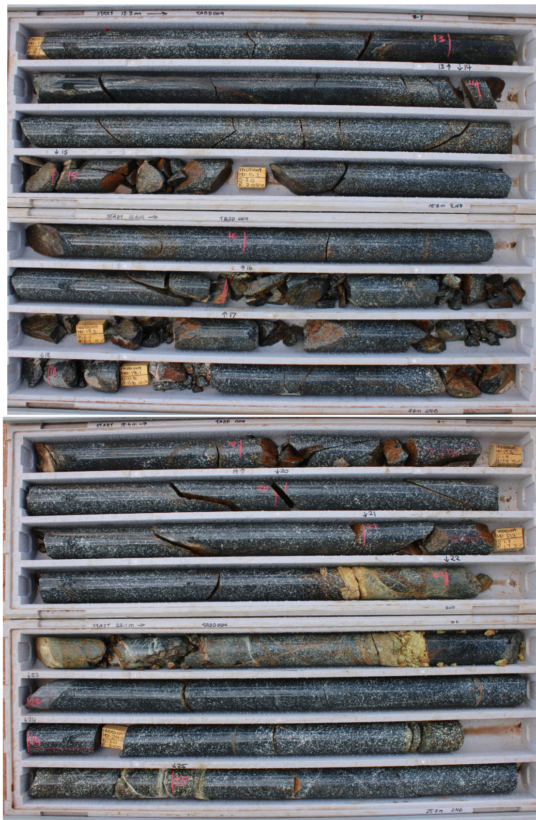
Plate I-4 (cont.): Unsaturated geological sequence at site TADD009 (0 to 25 m below ground level), located north the of the deposit.
