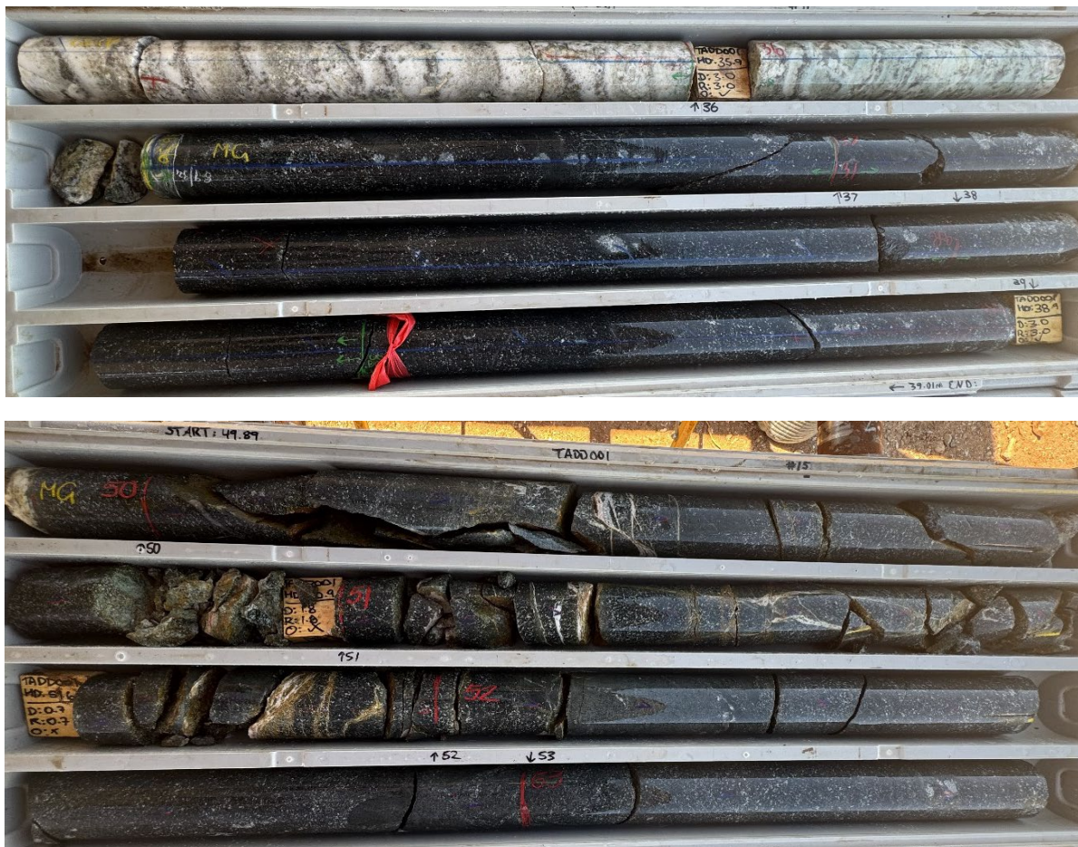
Plate II-1: Saturated geological sequence at site TADD001 showing the contact at the dolerite dyke (35.4 to 39 m bgl), and significant fracturing (water bearing) lower at 49.9 to 53.5 m bgl.
