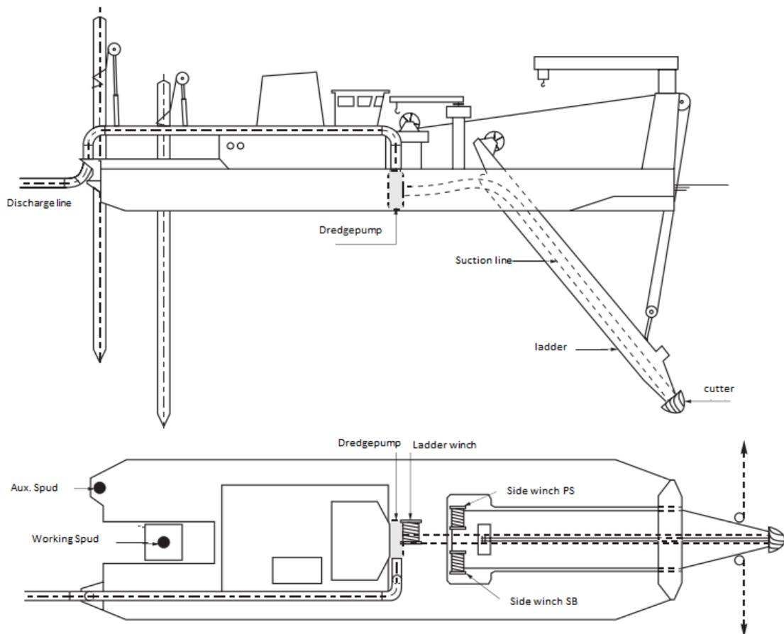
**Figure 3 Cutter Suction Dredge schematic**
