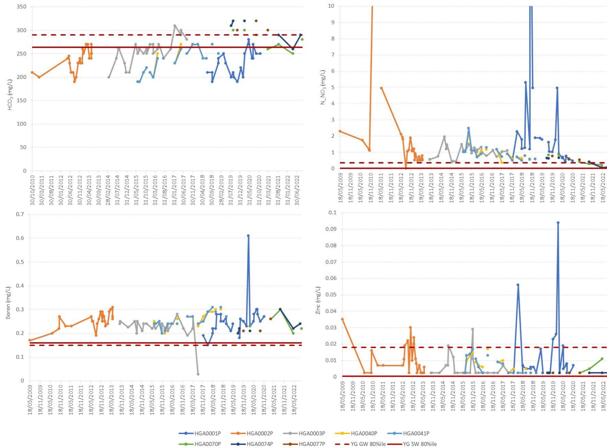
Figure 5.6: Time series plots of HCO 3 , N-NO 3 , dissolved boron and dissolved zinc from MAC groundwater monitoring bores, compared to YG 20%iles (pH)/80%iles
