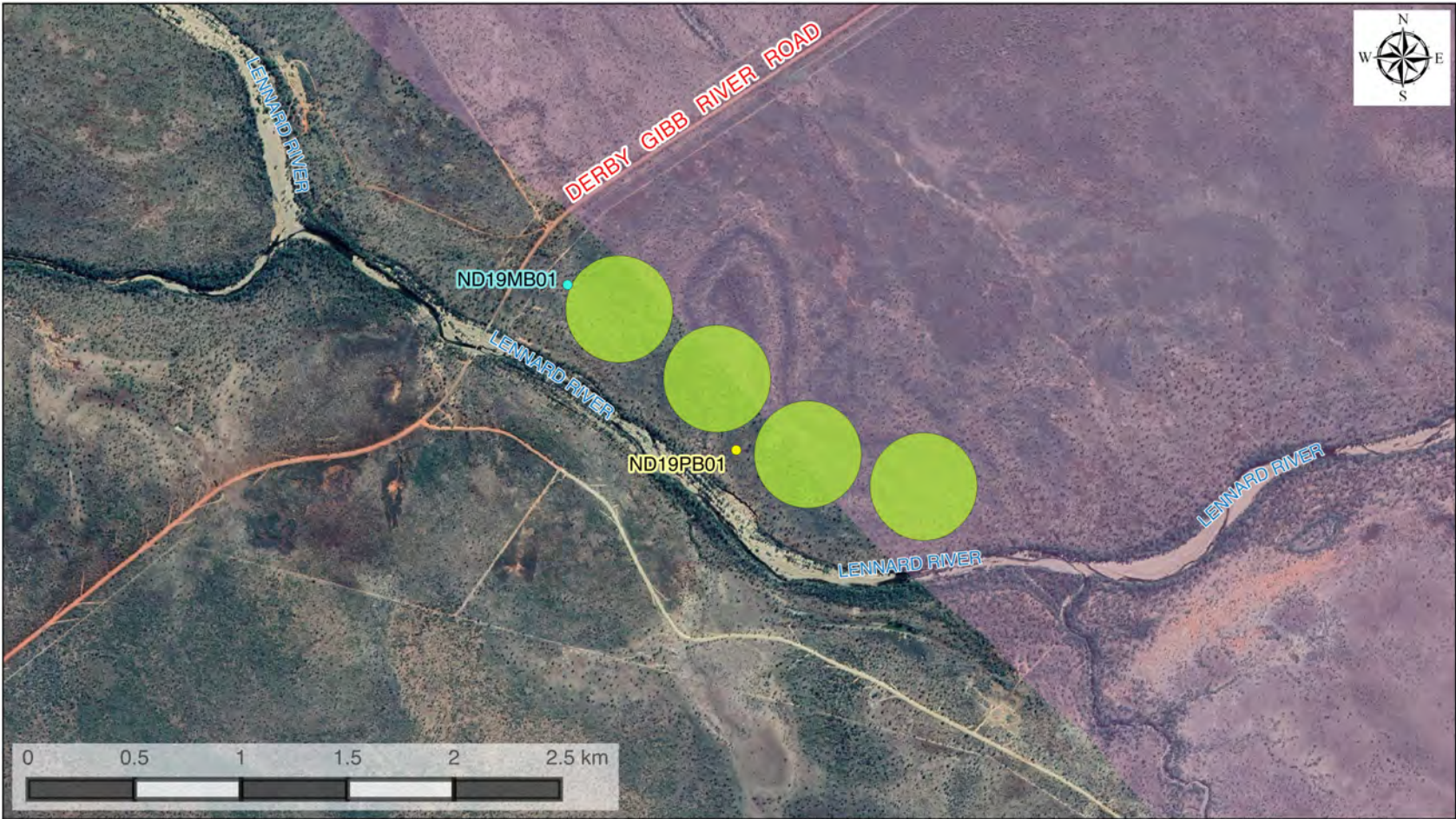
FIGURE 1. Location of recently drilled monitoring bore (ND19MB01) and proposed trial production bore (ND19PB01) as well as four proposed 20-hectare pivots for Stage 1 irrigation development. Note proximity to low-permeability Fairfield Group geology as shown by pale pink overlay.
