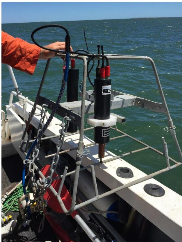
Figure 4a Water quality instruments mounted on the subsea frame from the WQMS.
