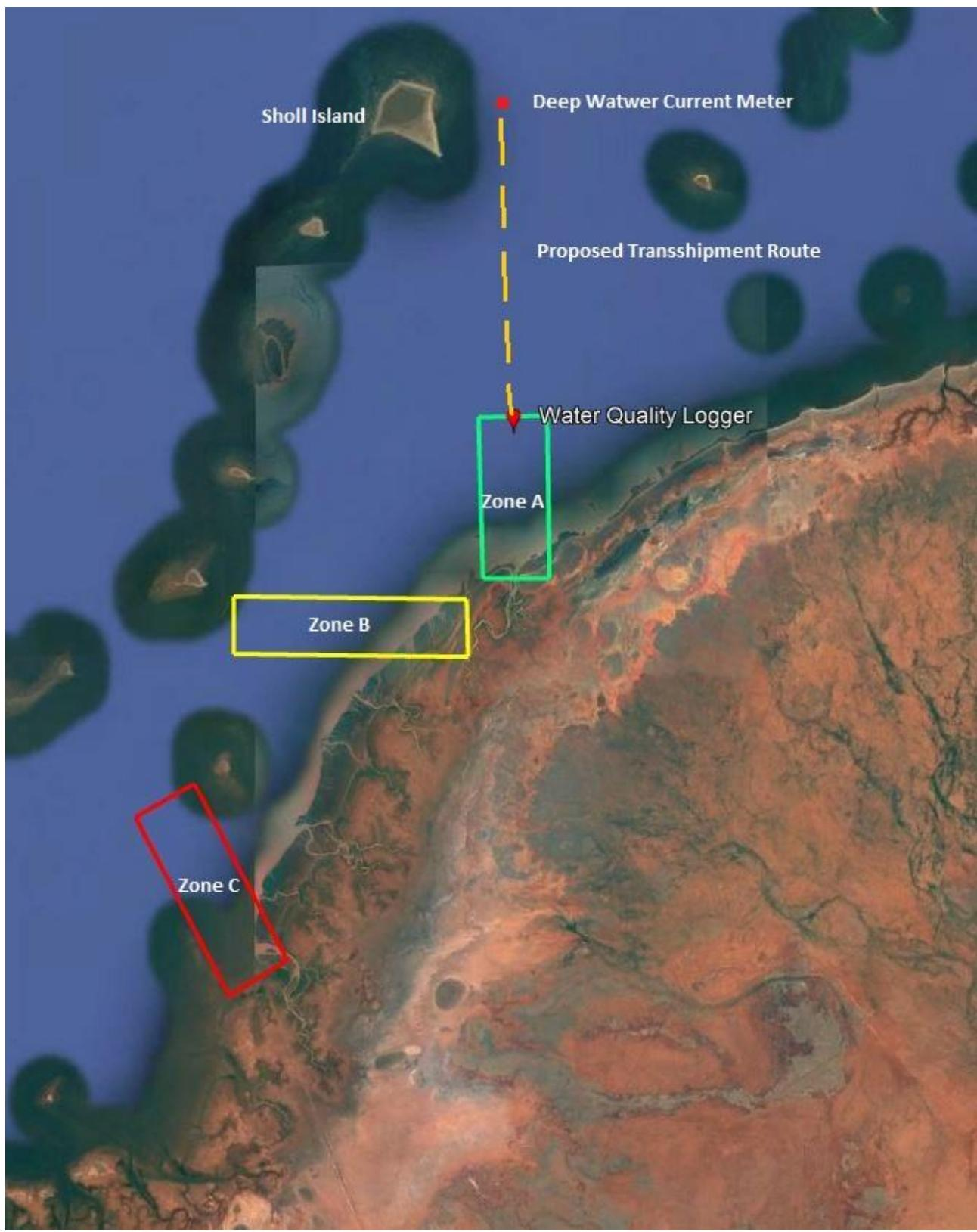
**Figure 1 Benthic Habitat Assessment Zones A, B and C, water quality instrument position and proposed transhipment route.**
