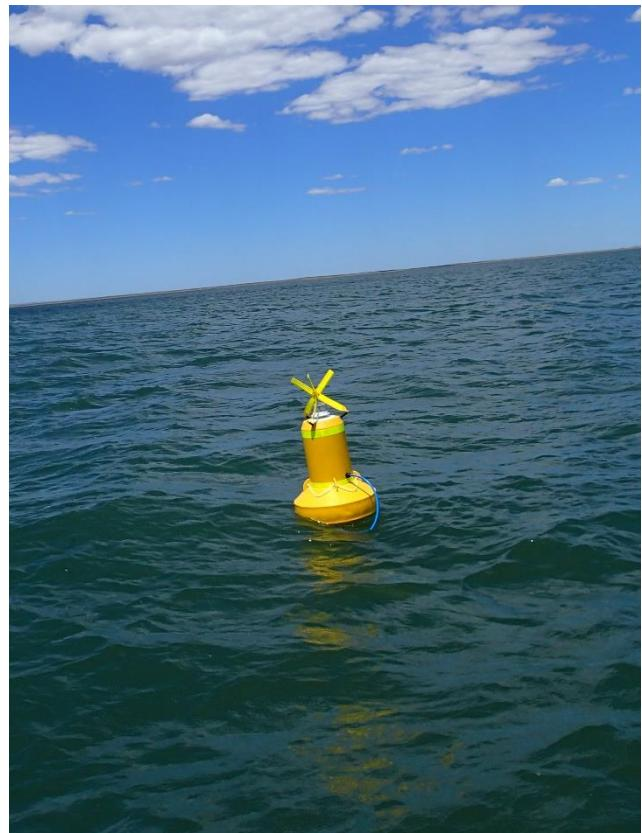
Figure 4b Surface buoy, navigation light and communication cables from the WQMS following deployment.
