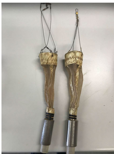
Figure 4 Stygofauna nets of different diameters showing the machined brass weight fitted to the bottom of the net and McCartney vial, with mesh base, that fits into the brass weight [58] (photo provided by Stantec)
