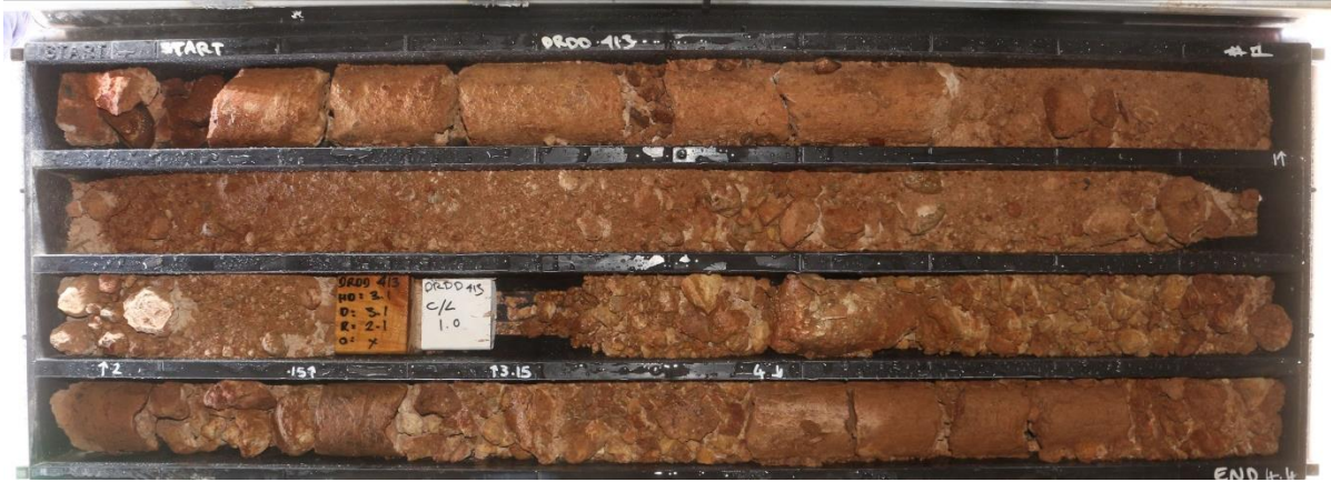
Plate 2 Clay dominated non-saturated zones or unfractured volcanic strata (Plate 1) shows Low or Nil troglofauna habitat potential.
