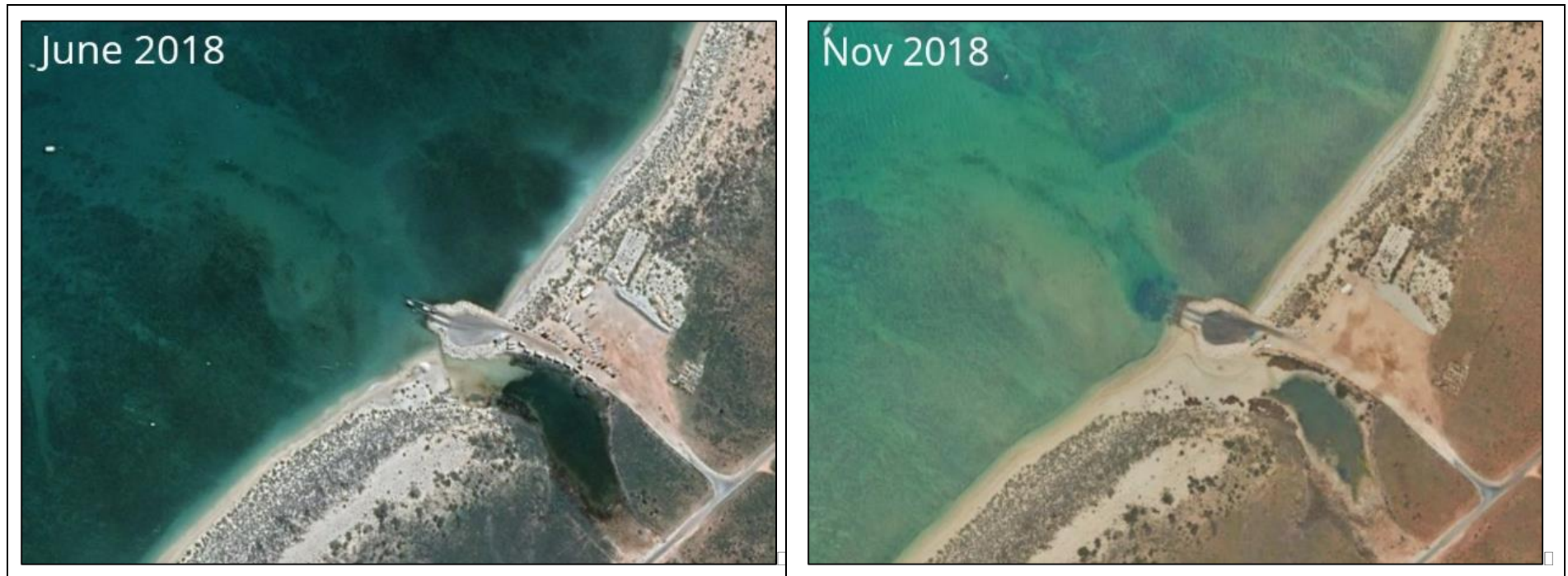
Figure 8-5. Aerial imagery showing the estuarine and coastal conditions immediately prior to the heaviest rainfall event of the year (June 2018) and five months after the rainfall event (November 2018). It is evident that the small-moderate rainfall event that occurred resulted in increased deposition of the sand bar but did not affect the navigability of the channel from the boat ramp. The November 2018 imagery suggests dredging may have occurred at the boat ramp as localised depression is evident. Image Credit: Google Earth and Landgate 2020
