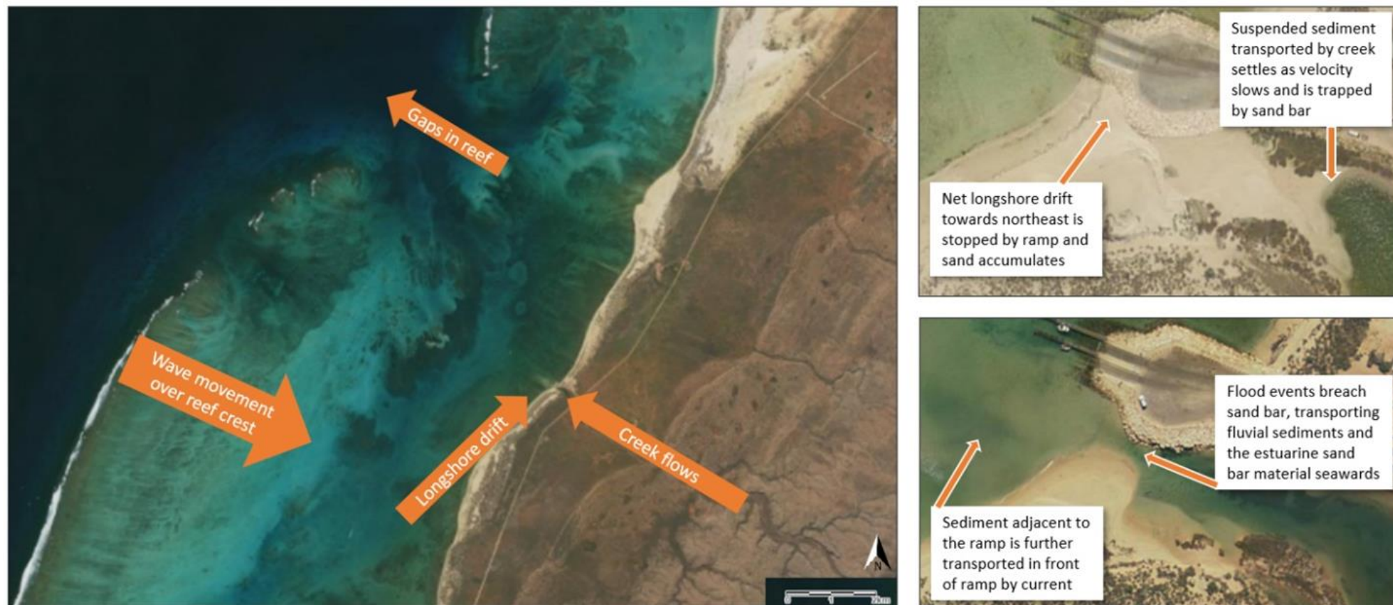
Figure 8-18. Sediment transport pathways at Tantabiddi Boat Ramp. a) General influences on sediment movement; b) Example of a small-moderate sized creek flow (e.g. 2018); c) Example of a larger creek flow (e.g. 2014). Imagery sourced from Landgate and Google Earth)
