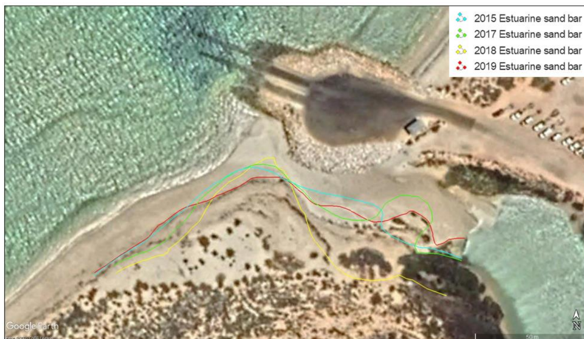
Figure 8-16. Estuarine sand bar changes from 2015 to 2019 based on extent of the northern berm of the sand bar. Note the lines do not show the extent of the exposed sand as this is subject to tidal variation (Source: Google Earth and Landgate).
