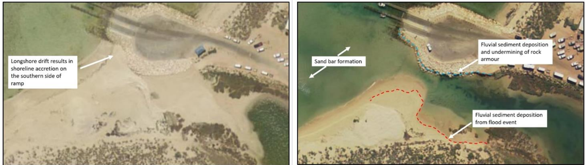
Figure 8-7. Sediment deposition from 2014 flood. Left: September 2013 prior to flood, shows clear sand bar and little evidence of red sediment from the upper catchment. Sand accretion has occurred along the south ramp. Right: July 2014 (after the April 2014 flood) shows red fluvial sediment lines on the sand bar (red line) and revetment (blue line) indicating flood extent. Sand bars and suspended sediment is present in the coastal waters to the south of the ramp and appear to cause waves to break over them.
