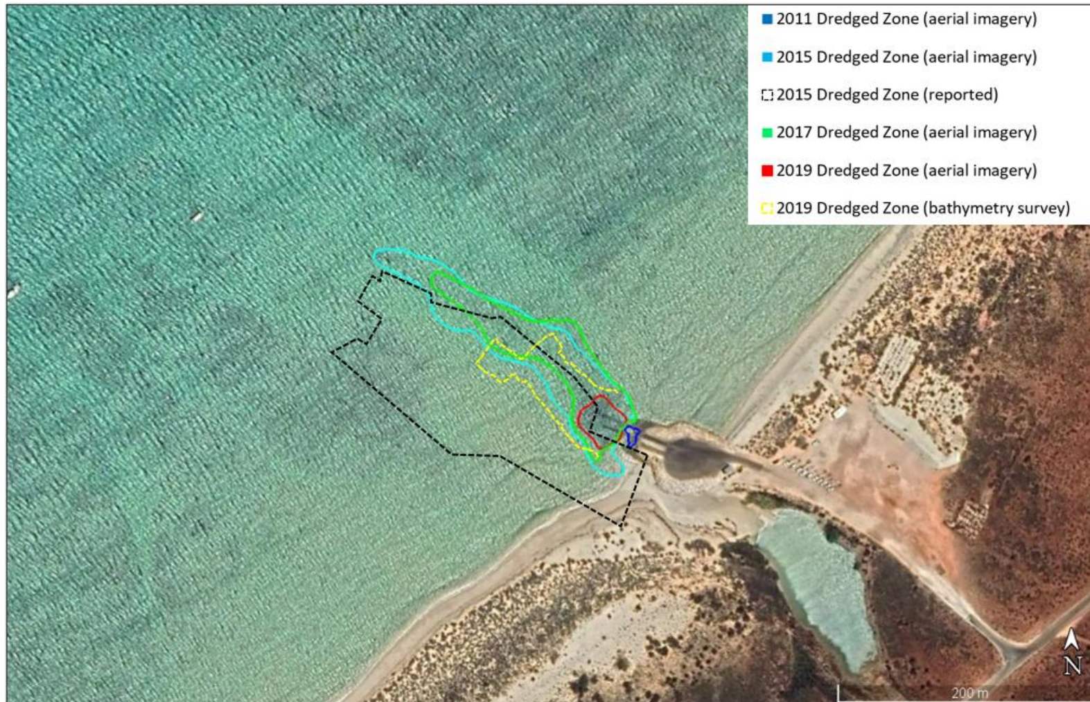
Figure 2-1. Dredged or excavated areas at the Tantabiddi Boat Ramp based on bathymetry, reports and aerial imagery from 2011 to 2019. Note: aerial imagery and bathymetric surveys were not conducted at the same time. Aerial imagery provides only an approximate estimate of dredge extent. Base imagery: November 2019.
