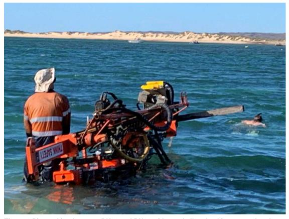
Figure 6 Rig tracking between BH02 and BH03 with snorkeller checking route ahead
