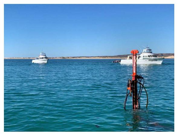
Figure 4 Subsea rig set up and ready to drill in boat mooring area at BH10
