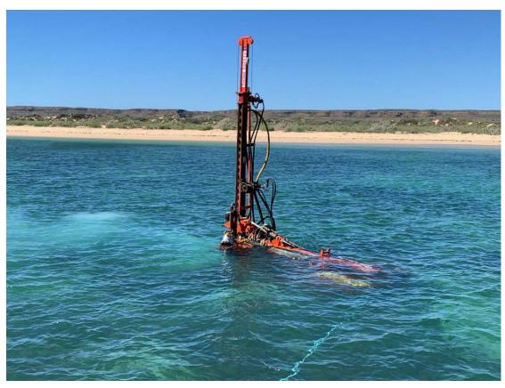
Figure 1 Subsea rig operating at BH01
