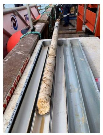
Figure 3 Limestone core transferred from core barrel in preparation for logging
