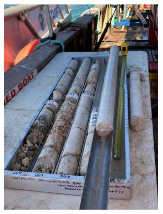
Figure 2 Calcisiltites (limestone) following extrusion from core barrel being prepared for logging
