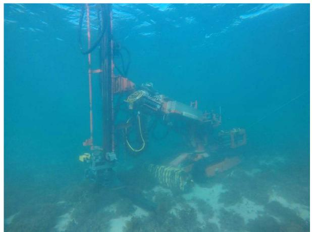
Diver/ driller recovering core barrel from subsea rig at BH12.
