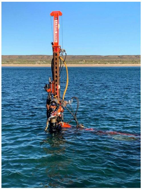
Figure 3 Diver/ driller recovering core barrel from subsea rig at BH12
