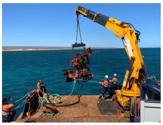
Figure 1 Overboarding subsea rig from the AMS Boss
