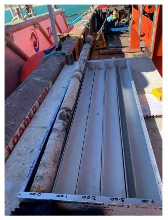
Figure 2 Limestone transferred from core barrel and prepared for logging
