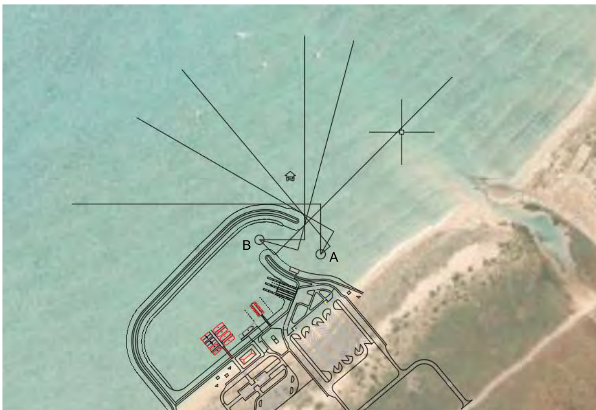
Figure 11.3 Wave Penetration Diagram for Concept B
