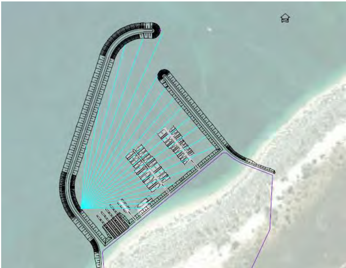
Figure 11.5 Example of Radial Fetch Length Calculation Concept C
