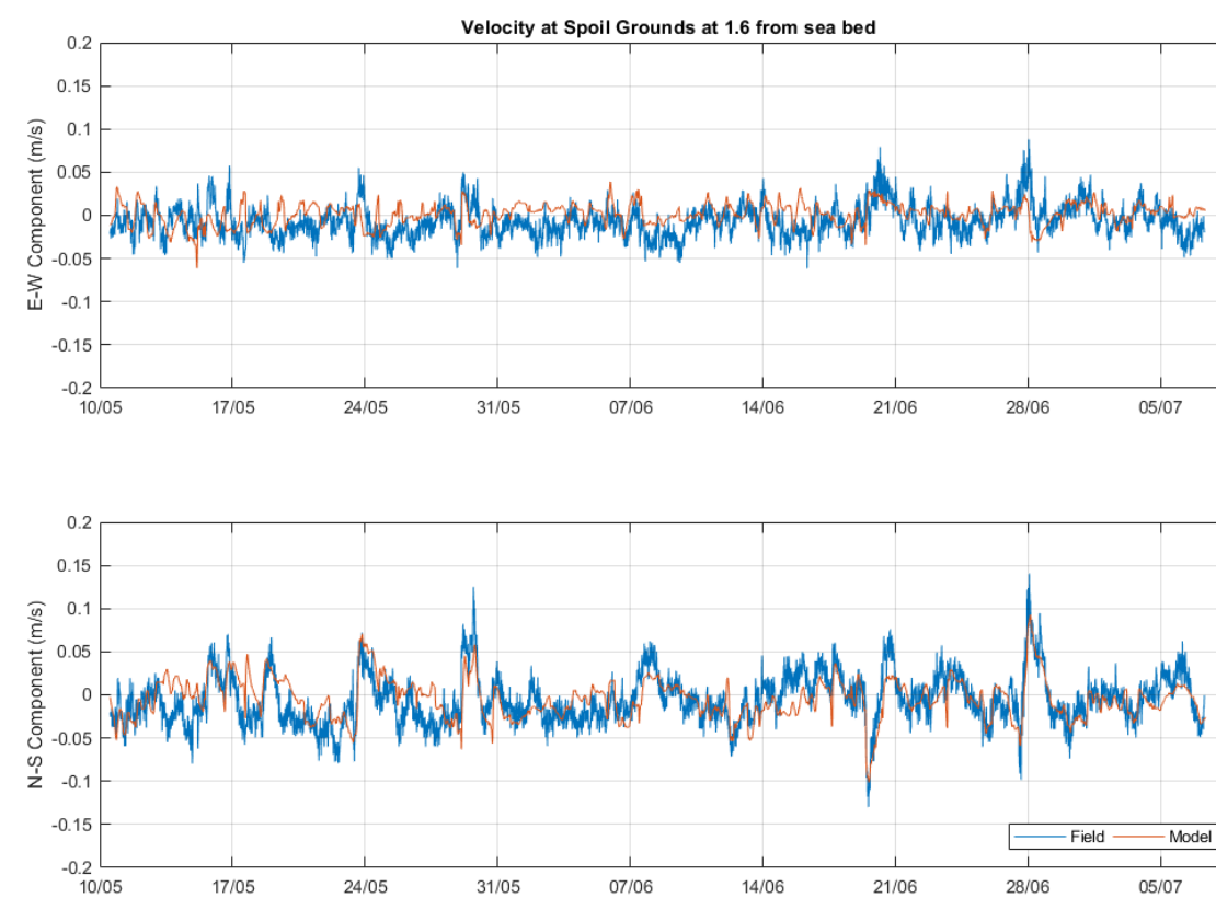
Figure 5-10 Comparison between simulated and measured ADCP velocities at 1.6m from sea bed at Spoil Grounds for May to July 2006
