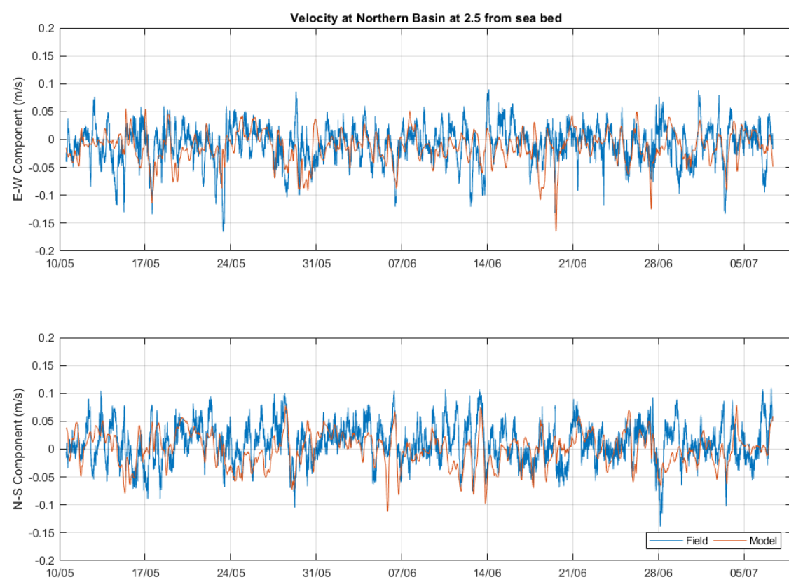
Figure 5-14 Comparison between simulated and measured ADCP velocities at 2.5m from the sea bed at Northern Basin for May to July 2006
