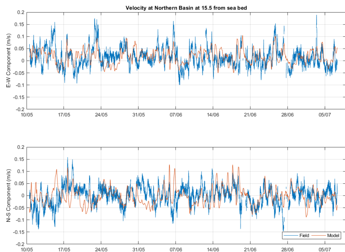
Figure 5-12 Comparison between simulated and measured ADCP velocities at 15.5m from the sea bed at Northern Basin for May to July 2006
