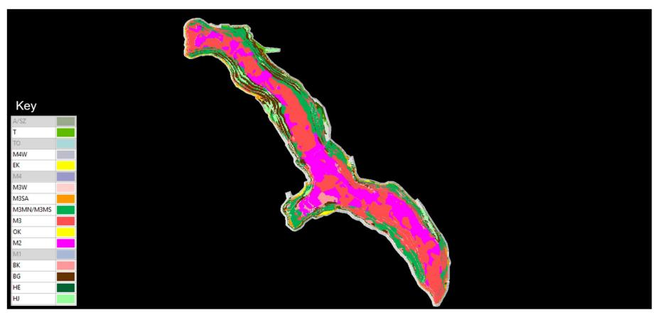
Figure J11. Stratigraphy of the E2/3/4/5/6 pit surface. Note that this intersection was created using two mining models (E2 and E23456) to achieve full coverage of the pit.
