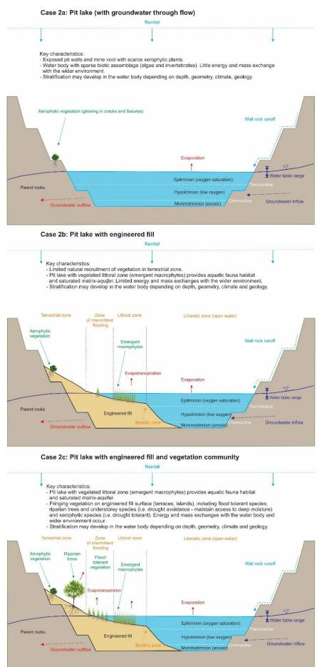
Figure F-2. Conceptual mine void closure option - Case 2 void includes a throughflow pit lake
