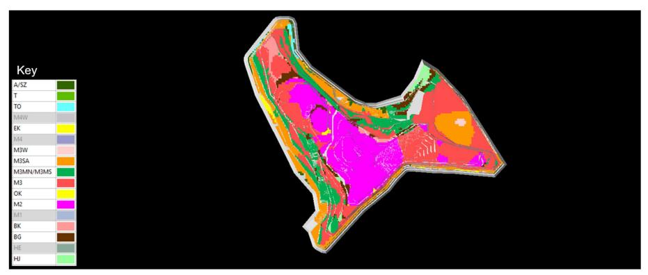
Figure J7. Stratigraphy of the W6 pit surface. Note that the intersection was created with two different mining models (C1C2 and W5678) to achieve full coverage of the pit.
