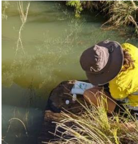
Plate 3.1: Filtering dissolved metal samples at MUNJS (photograph by Biologic ©).
