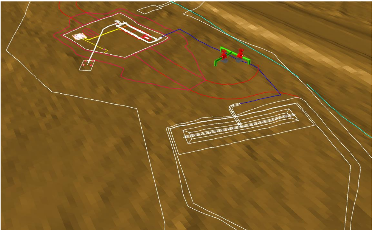
Figure 6-1 – Piping offtake to Aeration Ponds
