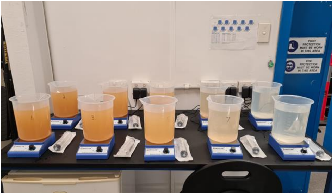
Figure 2-2 Batch 1 water samples showing heavy staining with iron oxyhydroxides. Beakers 1+2 = 100% OB32 (far left), beakers 3+4 = 90% OB32-10%OPD, beakers 5+6 = 50% OB32-50%OPD (middle), beakers 7+8 = 10%OB32-90%OPD, and beakers 9+10 = 100% OPD.
