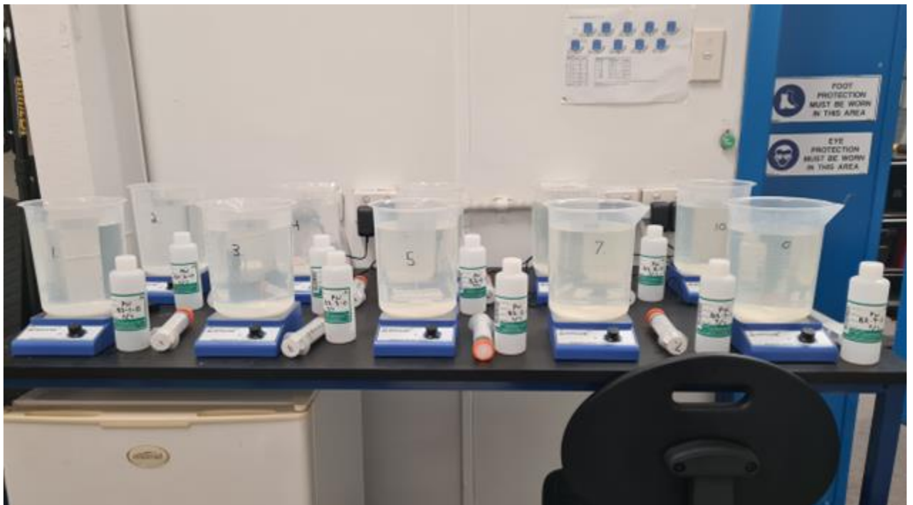
Figure 2-3 Batch 2 field filtered water samples. Beakers 1+2 = 100% OB32 (far left), beakers 3+4 = 90% OB32-10%OPD, beakers 5+6 = 50% OB32-50%OPD (middle), beakers 7+8 = 10%OB32-90%OPD, and beakers 9+10 = 100% OPD.
