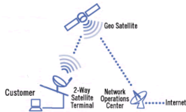
Two-way connection to the internet via satellite [39]
