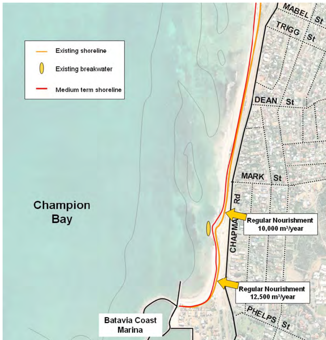
Figure 4-4 Medium term shoreline evolution for the present situation of the NSBP and an additional nourishment north of the detached breakwater
