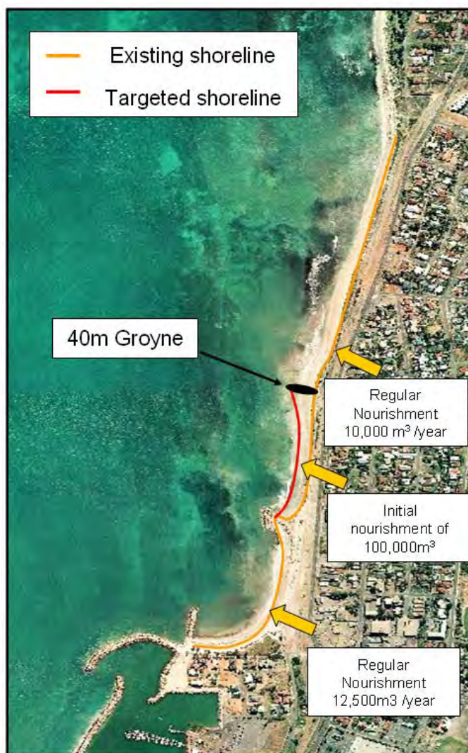
Figure 4-6 Possible coastal protection north of the breakwater (40m groyne)
