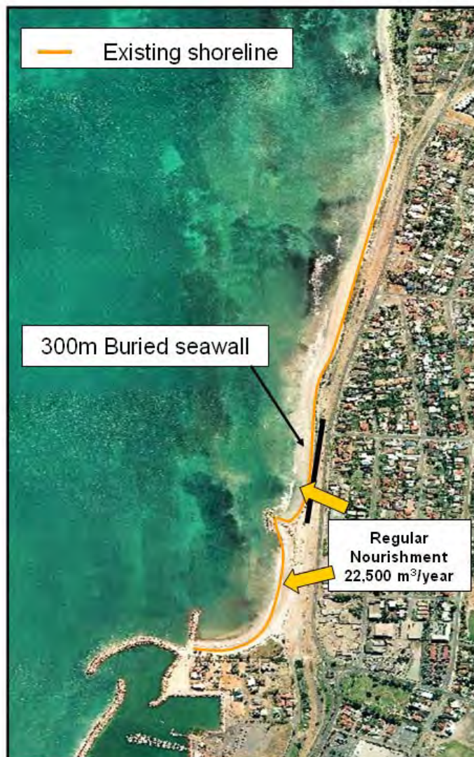
Figure 4-5 Possible coastal protection north of the breakwater (300m buried seawall)
