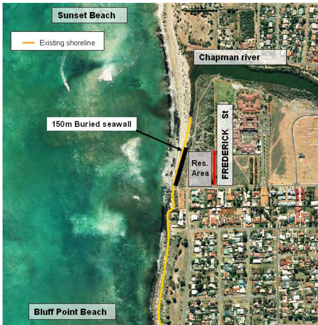
Figure 4-9 Possible coastal protection south of the Chapman river
