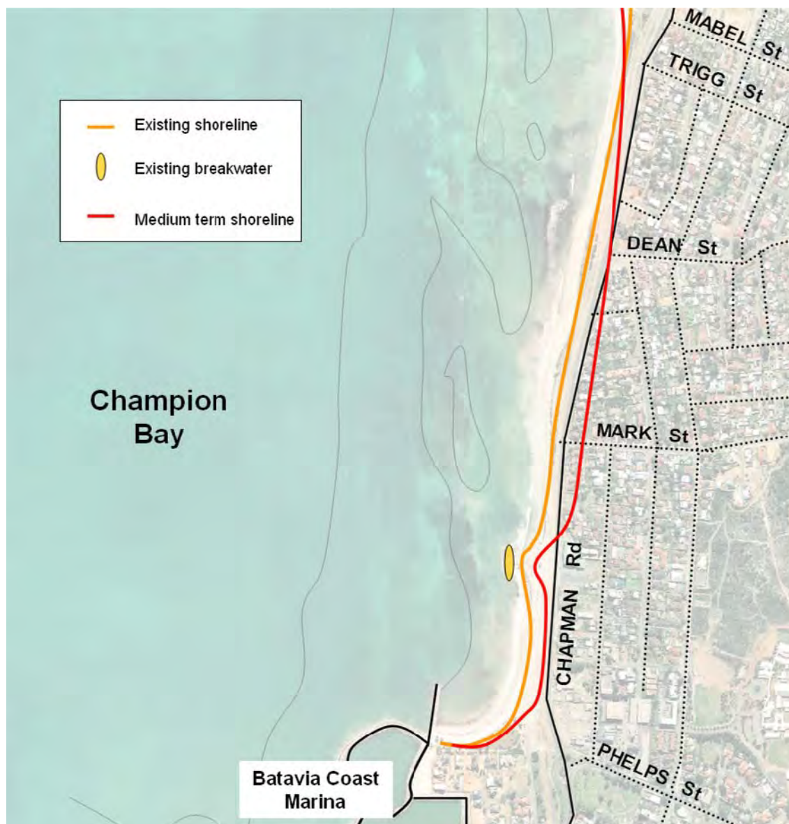
Figure 4-1 Medium term shoreline evolution for the case “Do Nothing” or “Managed Recession” along the Northern Beaches
