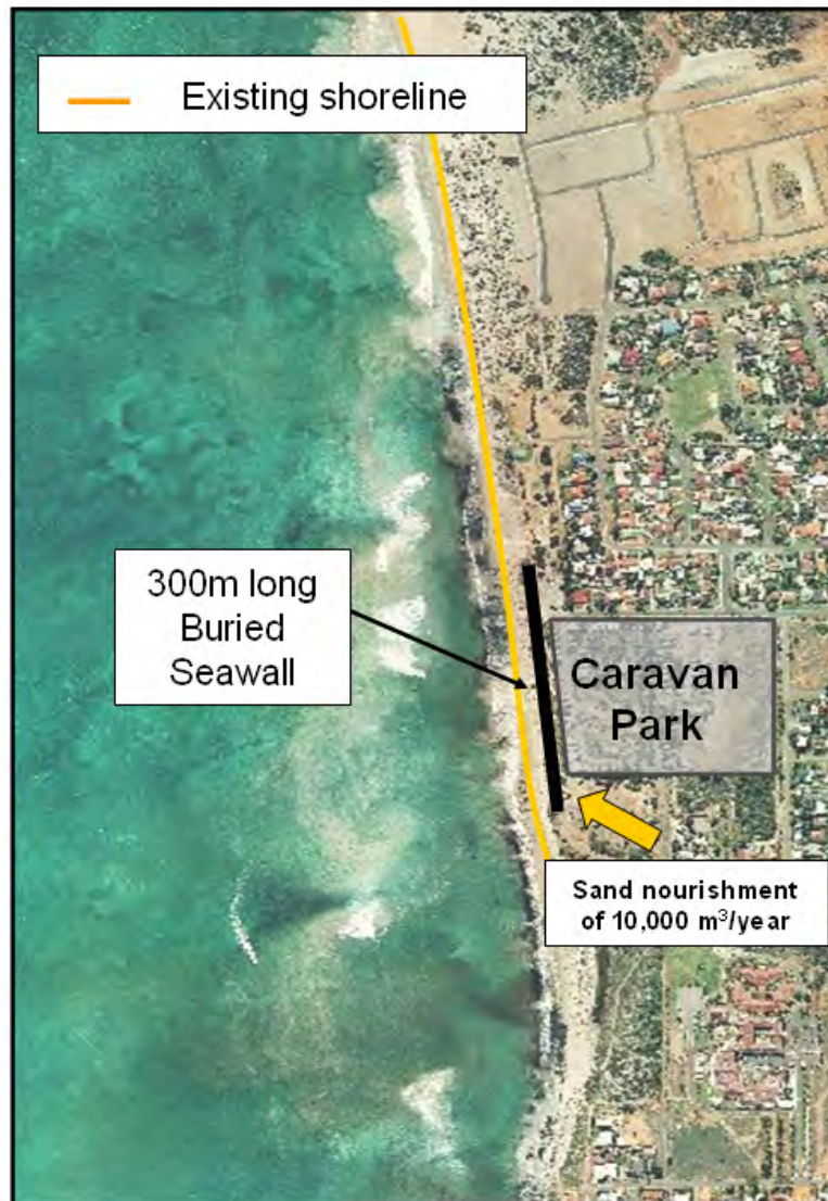
Figure 4-8 Possible coastal protection option at Sunset Beach
