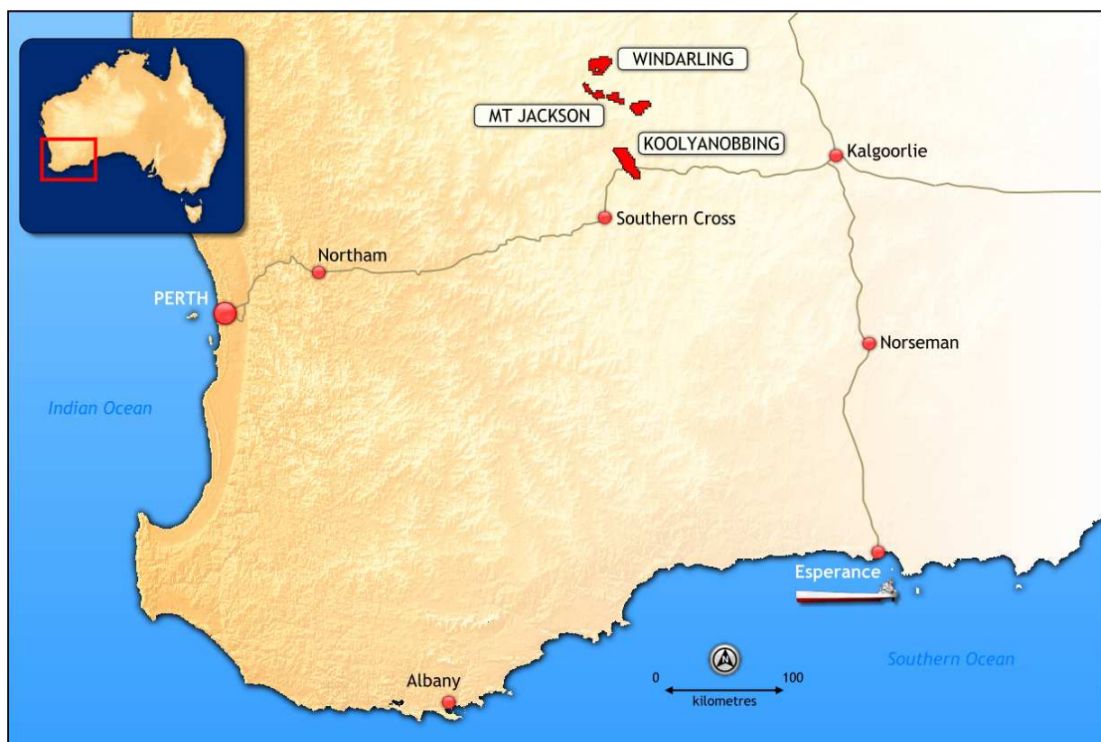
Figure 1-1 The Koolyanobbing Iron Ore Project. The Koolyanobbing Iron Ore Expansion Project involves mining of ore at Windarling, Mt Jackson and Koolyanobbing, with road transport of ore between the mines, and rail transport between the Koolyanobbing mine (via Kalgoorlie and Norseman) to Esperance where the ore is exported.
