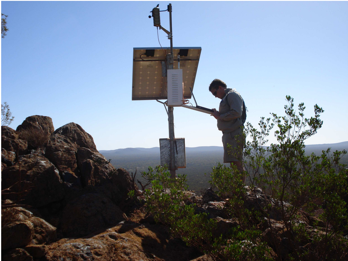
Figure 3-4 An Osiris dust monitor being checked near the Windarling W3/5 pit by an Environmental Officer in accordance with the approved Dust Management Plan.
