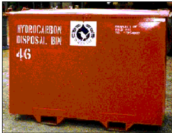
Hydrocarbon disposal bin (rags, hoses etc)
