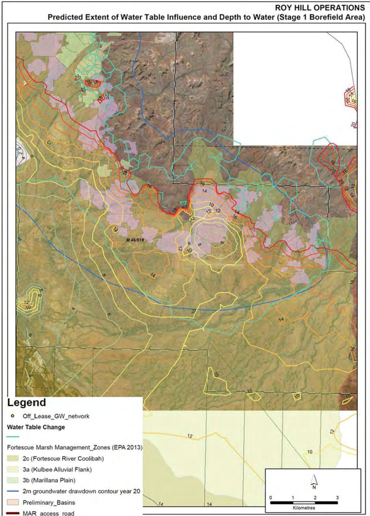
**Figure 13.** Depth to the watertable after two years of reinjection in the Stage 1 Borefield (Roy Hill 2018).
