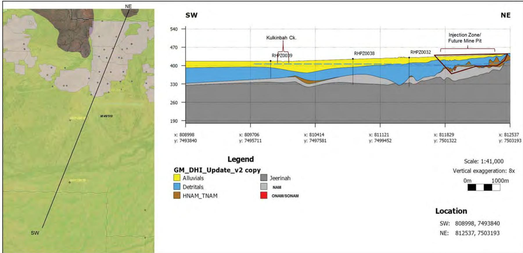
**Figure 6.** Cross-section of the Stage 1 Borefield (Roy Hill 2018).
