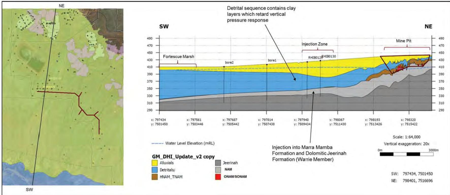
Figure 5. Cross-section of the SWIB (Roy Hill 2018).
