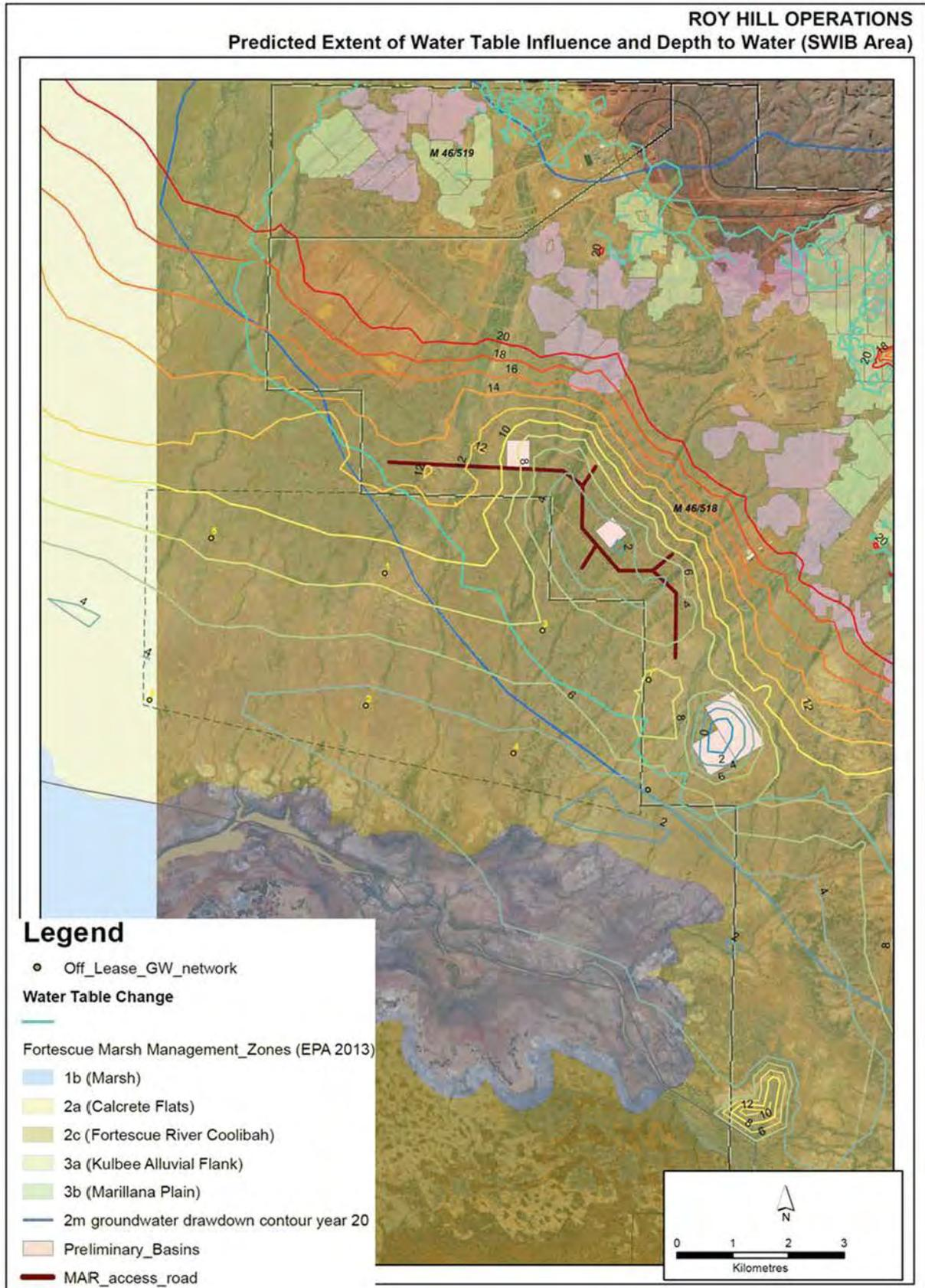
**Figure 12.** Depth to the watertable after two years of reinjection in the SWIB (Roy Hill 2018). Natural watertable at the injection site is 20 mbgl.
