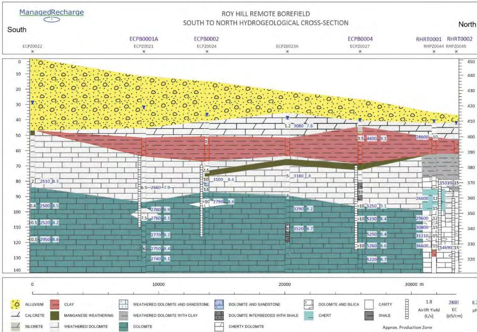
**Figure 7.** Cross-section of the Stage 2 Borefield (Managed Recharge 2018).
